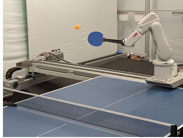
Figure 1: Robot setup An ABB IRB 120T 6-DOF robotic arm is mounted to a two-dimensional Festo linear actuator, creating an 8-DOF system.
