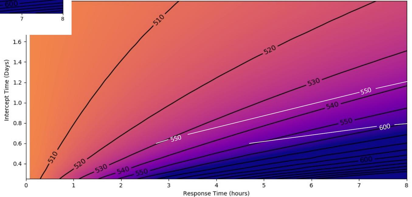
Alt/FPA target results in savings of ~10 m/s for this epoch compared to target line
