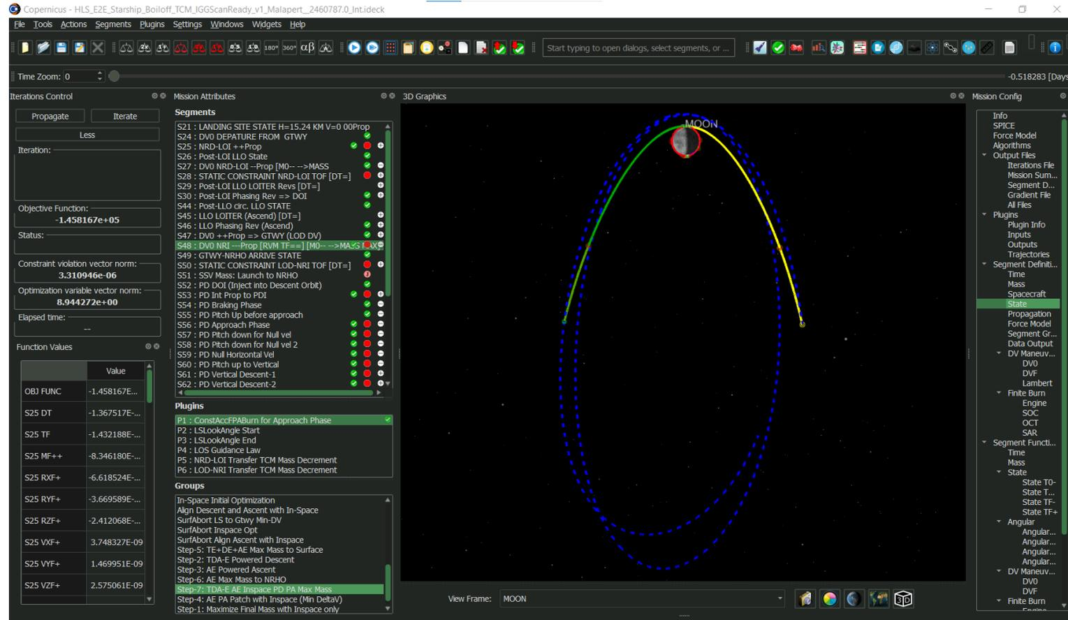
For HLS mission, Copernicus is used for minimizing In-space Delta-V and prop mass used for powered descent/ ascent, and for satisfying the mission-specific constraints simultaneously
