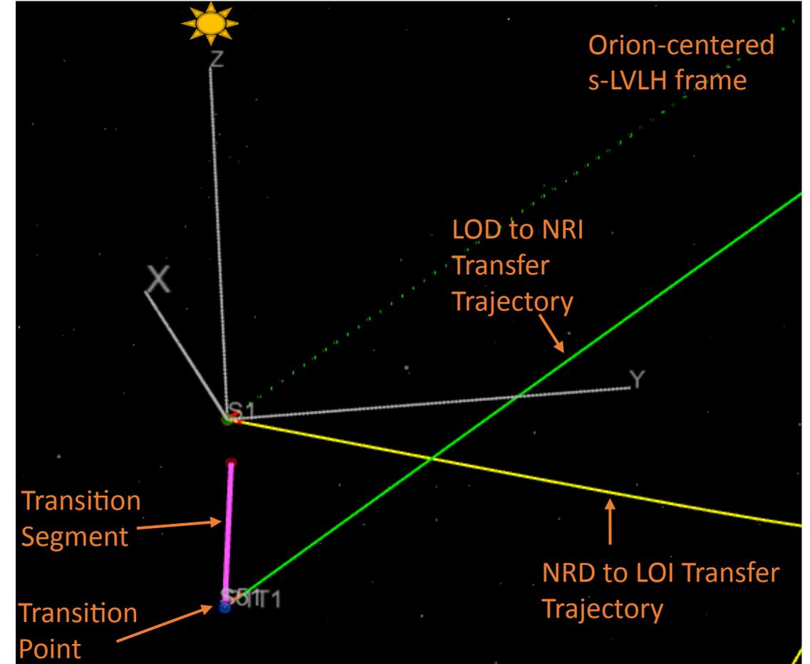
Depending on the mission epoch, HLS can approach the transition point from different directions
