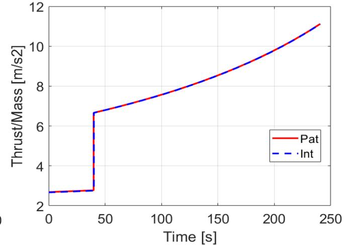
End-to-end optimized solution has almost the same performance as that of the patched sim.
