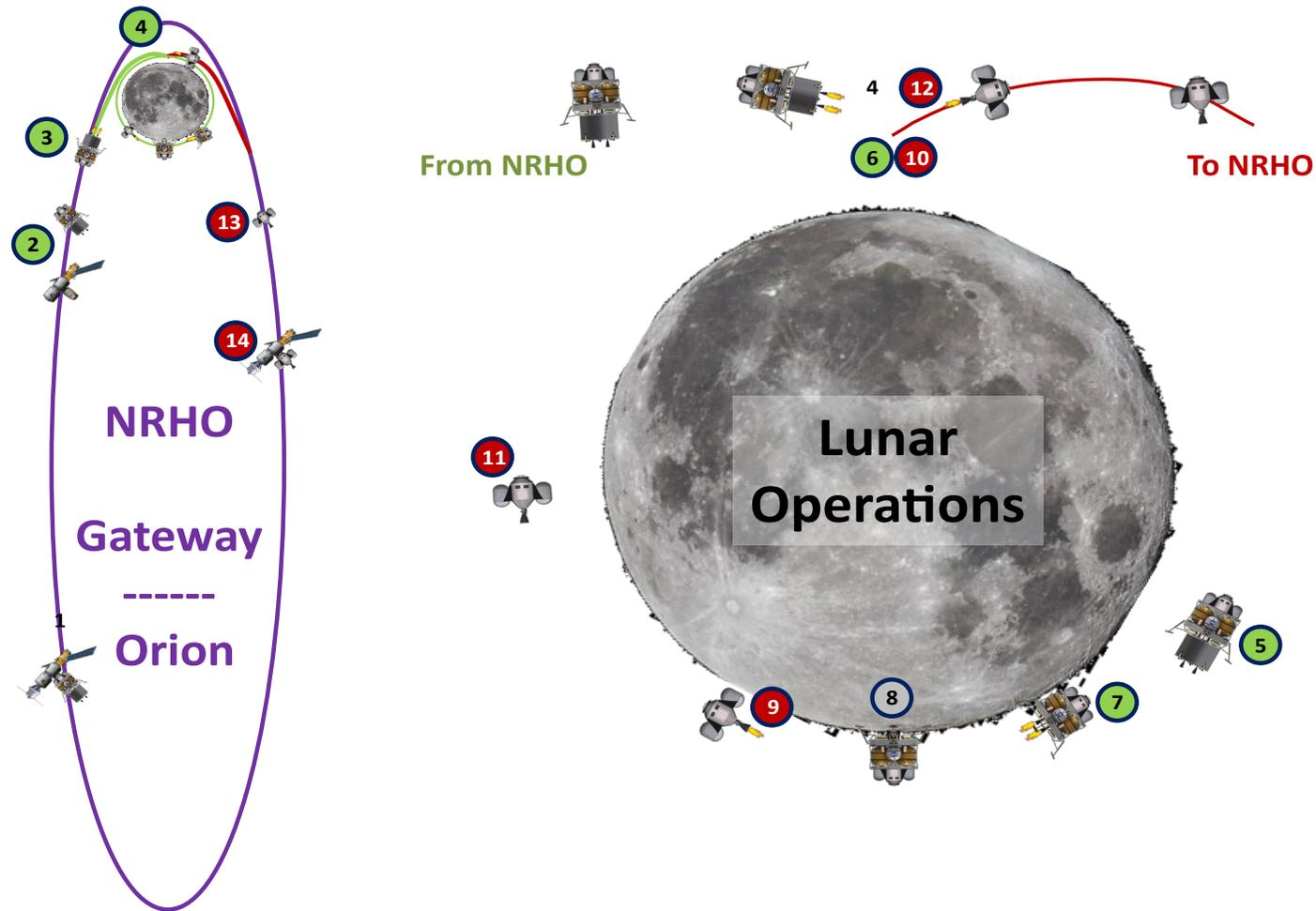
1. NRHO Gateway: 9:2 Lunar Synodic Resonant, ~6.5 day Orbit Period, HLS Lunar Lander Attached to Gateway / Orion
