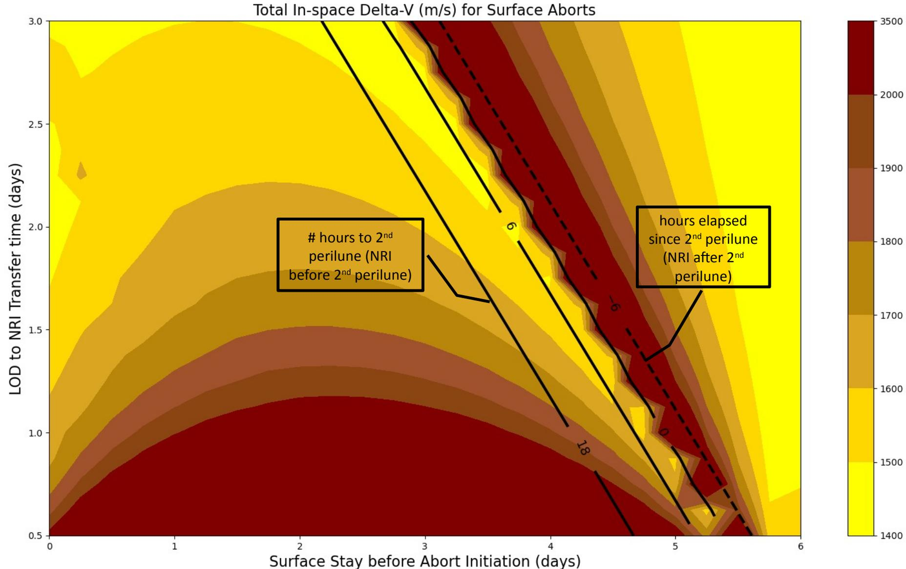
\*Surface stay time resolution = 6 hrs, LOD to NRI Transfer time resolution= 3 hrs
