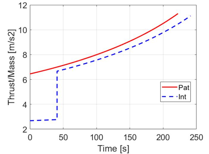
Powered ascent in the end-to-end optimized solution has longer duration by 20 sec than that of the patched sim and as a result, has lower prop mass usage by ~87 kg
