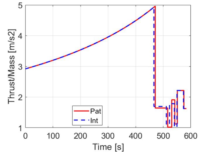
End-to-end optimized solution's PDI occurs at lower altitude than that of the patched sim and as a result, has better performance by ~80 kg of prop mass
