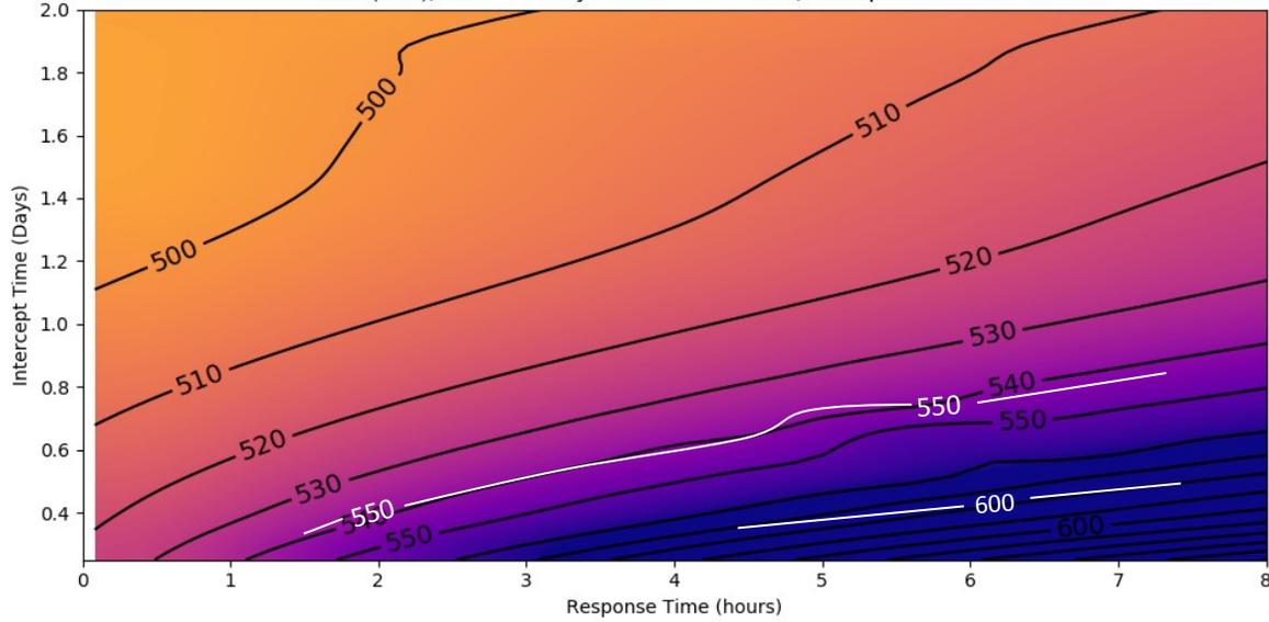
Orion-Assisted Abort (AE NRHI failure), Return to Earth to Target Line (44 crew-day limit on return), Total  $\Delta V$  (m/s) Ref Epoch: 16 Mar 2024
