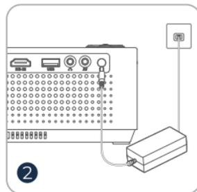
2 Connect the power adapter to an outlet.
