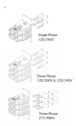
If you require different inserts or contacts for local code, WINCO has a variety of different inserts and contacts available. Contact the factory at 507-357-6831 for pricing.
