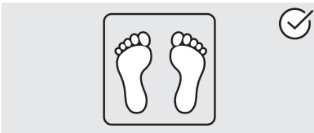
Measuring body fat and other body composition parameters correctly: stand straight on the scale, with both feet placed over the electrodes as shown in the above figure.
