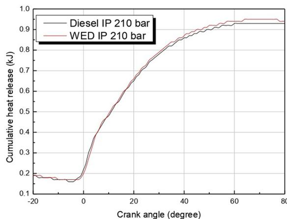
**Fig. 3** Variations of cumulative heat release with crank angle at injection pressure of 210 bar for base diesel and WED
