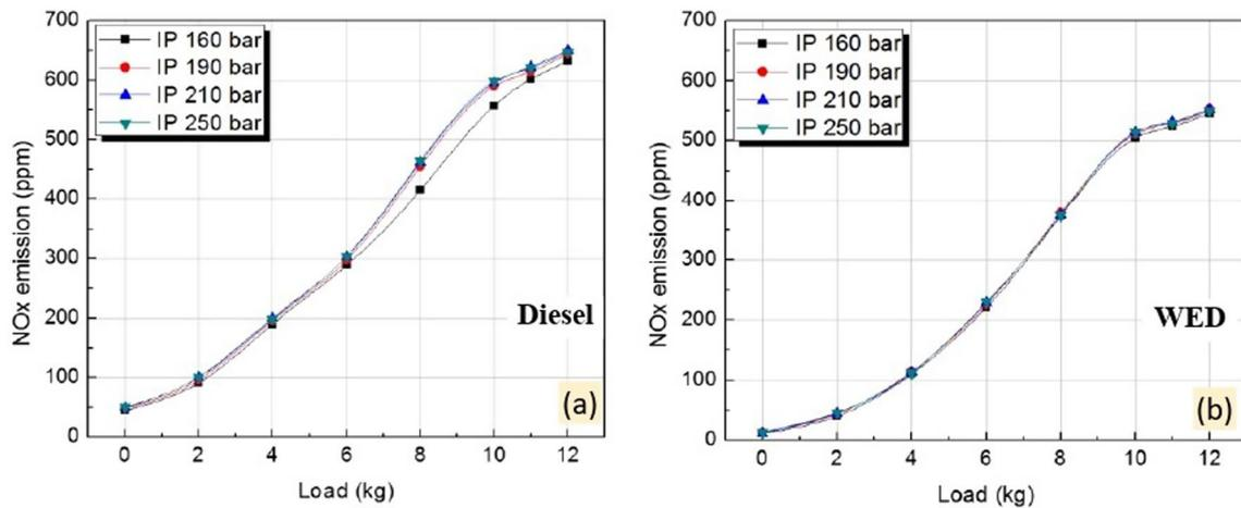
**Fig. 10** Variation of NO<sub>x</sub> emission with load at different injection pressures using **a** normal diesel and **b** WED
