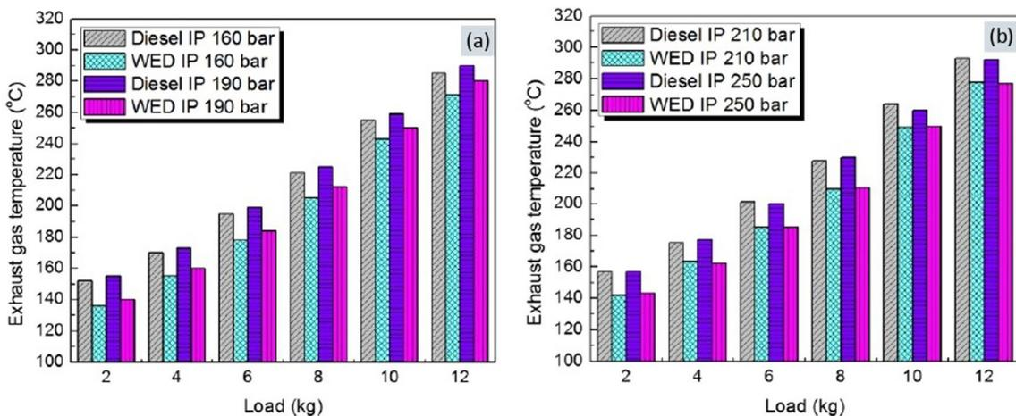
**Fig. 9** Variation of exhaust gas temperature with load at injection pressures of **a** 160 bar and 190 bar and **b** 210 bar and 250 bar for base diesel and WED
