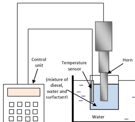
**Fig. 1** Schematic diagram of the Ultrasonicator
