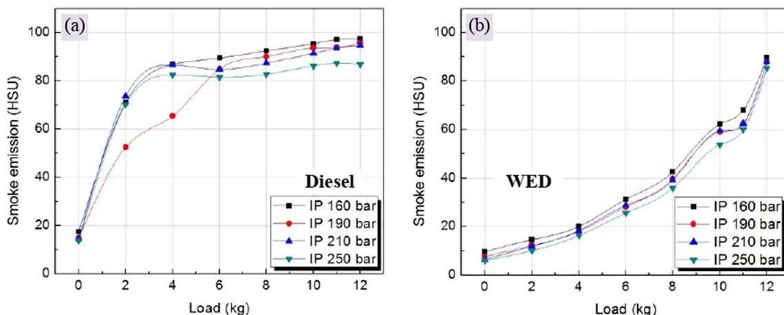
**Fig. 12** Variation of smoke emission with load at different injection pressures using **a** normal diesel and **b** WED
