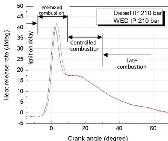
**Fig. 5** Comparison of the net heat release rate with crank angle using base diesel and WED
