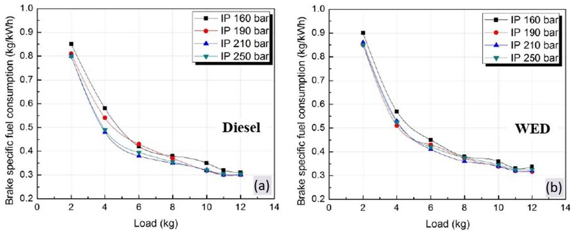
**Fig. 8** Variation of the BSFC with load at different injection pressures using **a** normal diesel and **b** WED
