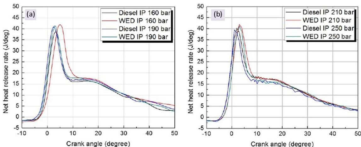
**Fig. 4** Variations of net heat release rate with crank angle at injection pressures of **a** 160 bar and 190 bar and **b** 210 bar and 250 bar for base diesel and WED
