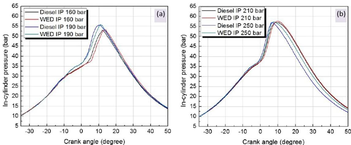
**Fig. 6** Variations of in-cylinder pressure with crank angle at injection pressures of **a** 160 bar and 190 bar and **b** 210 bar and 250 bar for neat diesel and WED
