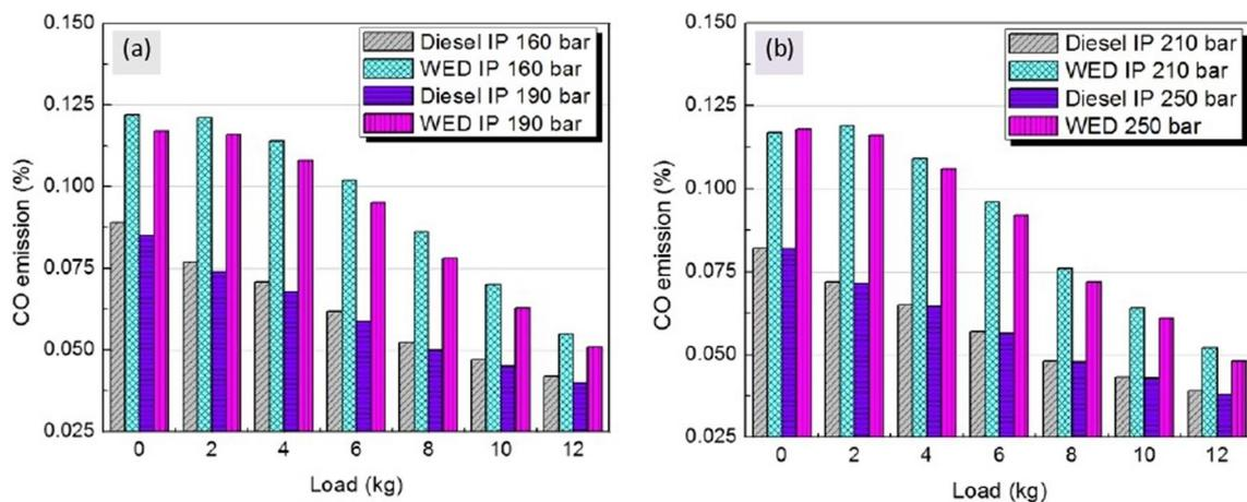
**Fig. 11** Variation of CO emission with load at injection pressures of **a** 160 bar and 190 bar and **b** 210 bar and 250 bar for base diesel and WED
