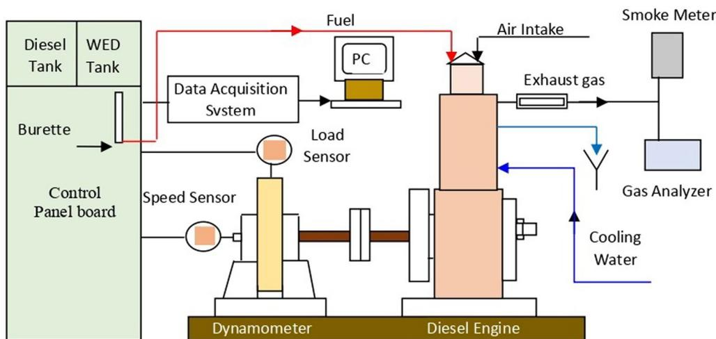
**Fig. 2** Schematic View of the Experimental Setup
