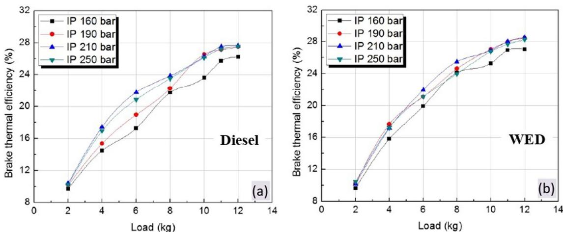
**Fig. 7** Variation of the brake thermal efficiency with load at different injection pressures using **a** normal diesel and **b** WED
