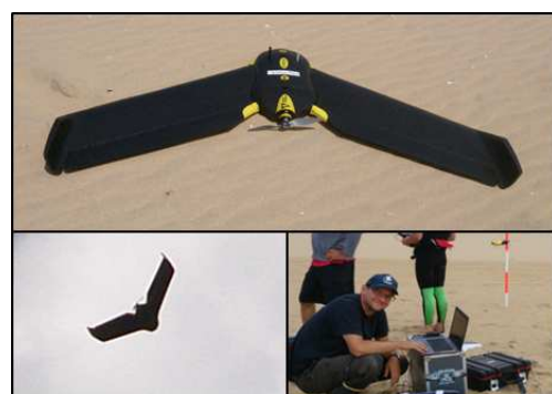
Figure 3. eBee UAV during a field campaign, in flight and the hardware
