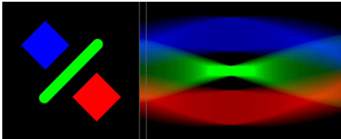
Horizontal projections through the shape result in an accumulated signal (middle bar). The sinogram on the right is generated by collecting many such projections as the shape rotates. Here, color is used to highlight which object is producing which part of the signal. Note how straight features, when aligned with the projection direction, result in stronger signals.
