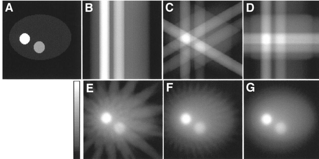
(A) Slice used to create projections. (B–G) 1, 3, 4, 16, 32, and 64 projections equally distributed over  $360^\circ$  are used to reconstruct slice using backprojection algorithm.
