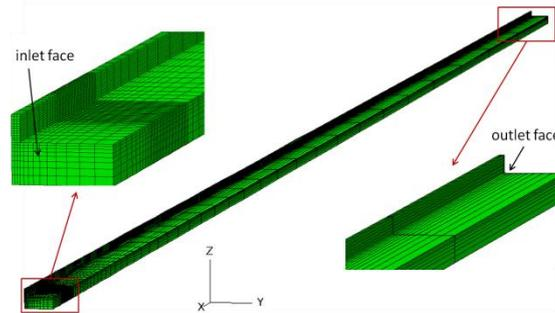
**Fig. 4: Mesh of the steady state thermal model.**
