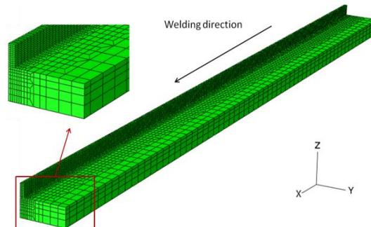
**Fig. 3: Mesh of transient thermal model.**
