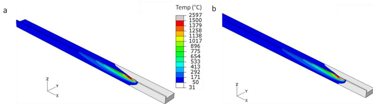
**Fig. 5: Temperature distribution from: (a) transient and (b) steady-state thermal models.**
