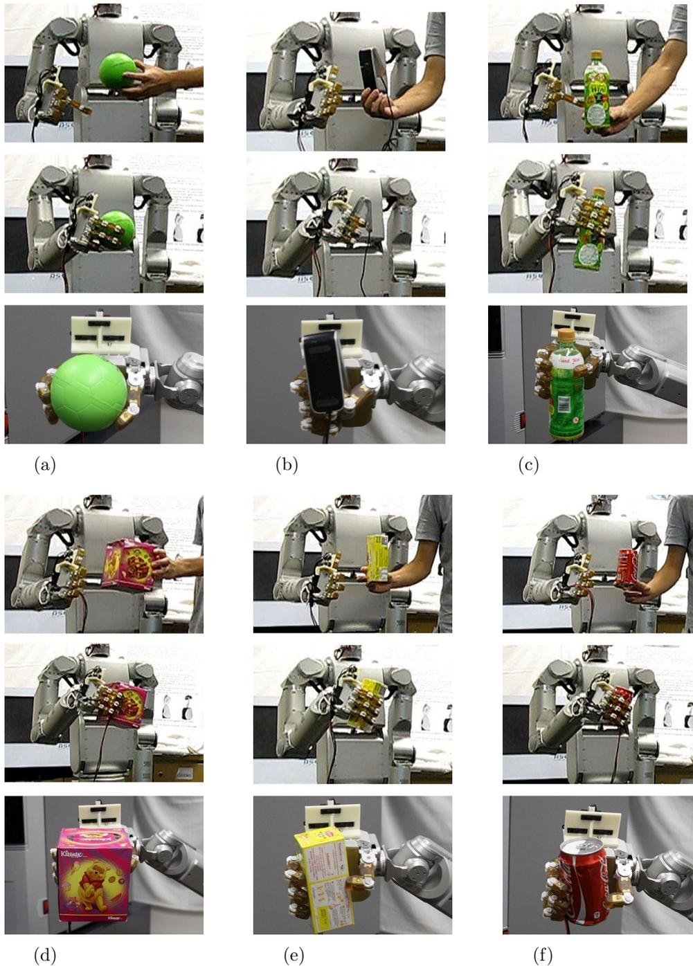
Figure A.1: Grasp experiments: for every object, the top picture shows the initial position of the sensor detecting an object. The middle and the bottom pictures show the final grasp from front view and side view respectively.
