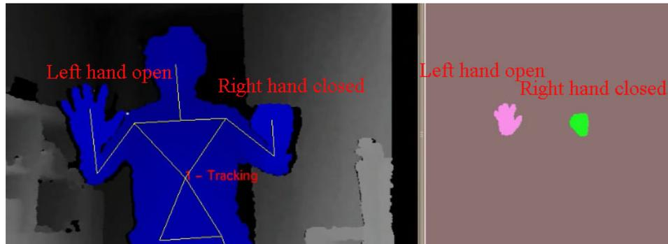
Figure 2.7: Hand detection. The right figure shows the hand detection result from the left figure.
