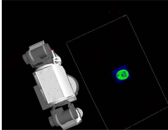
Figure 3.4: Simulation on RVIZ. It shows the detection of the table, the can, and the robot model. The blue cube indicates the selected object.
