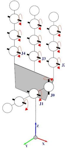
Figure 2.17: MEKA robotics hand joint names and directions: the posture shown 0 joint angles, arrows show positive rotation and torque directions [2]
