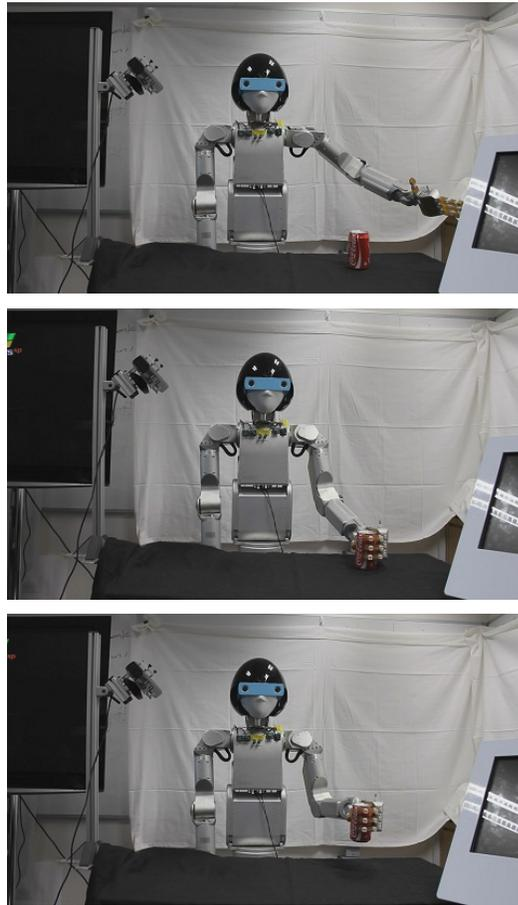
Figure 3.5: Autonomous grasping. The first image shows pre-grasp. The second image shows the robot hand wraps an object. The third image shows the robot lifts the object.
