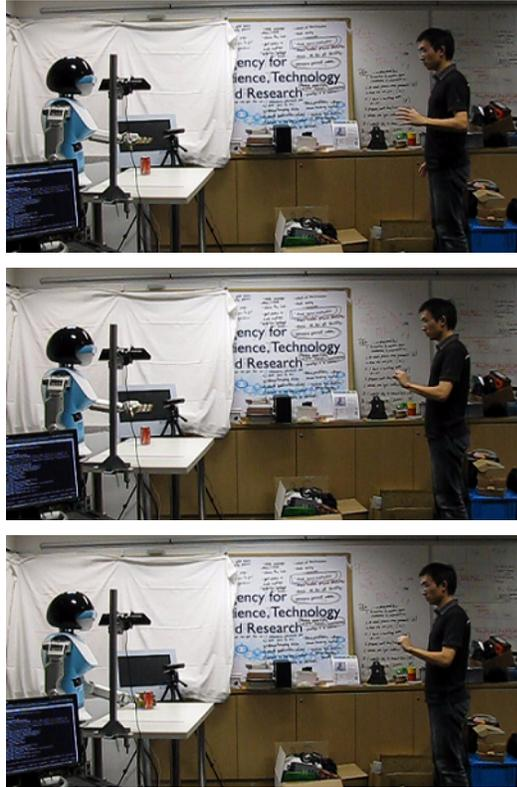
Figure 3.6: Grasping object using the combined method. The first image shows the teleoperation. The second image shows the switching from the teleoperation to autonomous grasping. The third image shows autonomous grasping.
