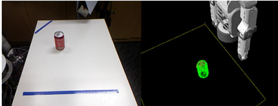
Figure 2.19: Table and object detection. The left image shows a table, a can and MEKA robot from Kinect RGB sensor. The right image shows the detection of the table and the can and robot model from RVIZ (A 3d visualization environment for robots using ROS) simulation.
