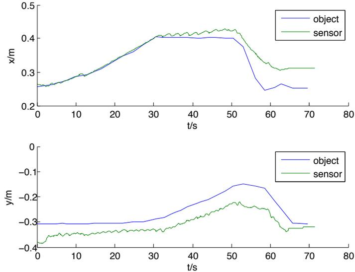
Figure 3.21: Trajectories of sensor 3 and the object during the tracking task
