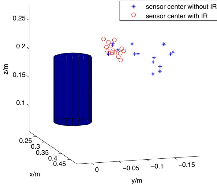
Figure 3.9: Teleoperation with and without the proposed IR Algorithm. The blue cylinder represents a soda can, and the points the pre-grasp positions.
