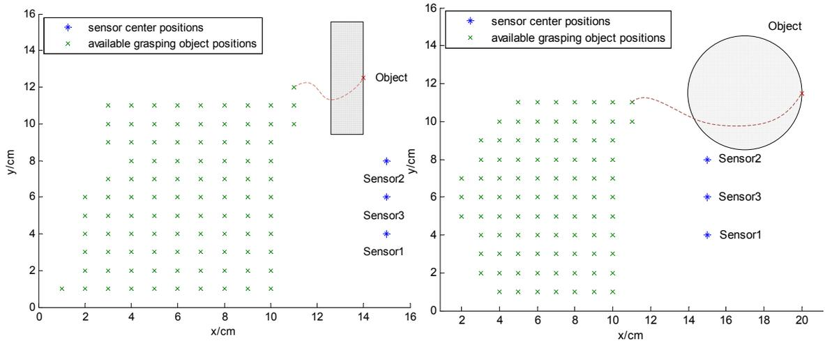
(a) Graspable area map of a sample object with rectangular cross-section. (b) Graspable area map of a sample object with circular cross-section.
