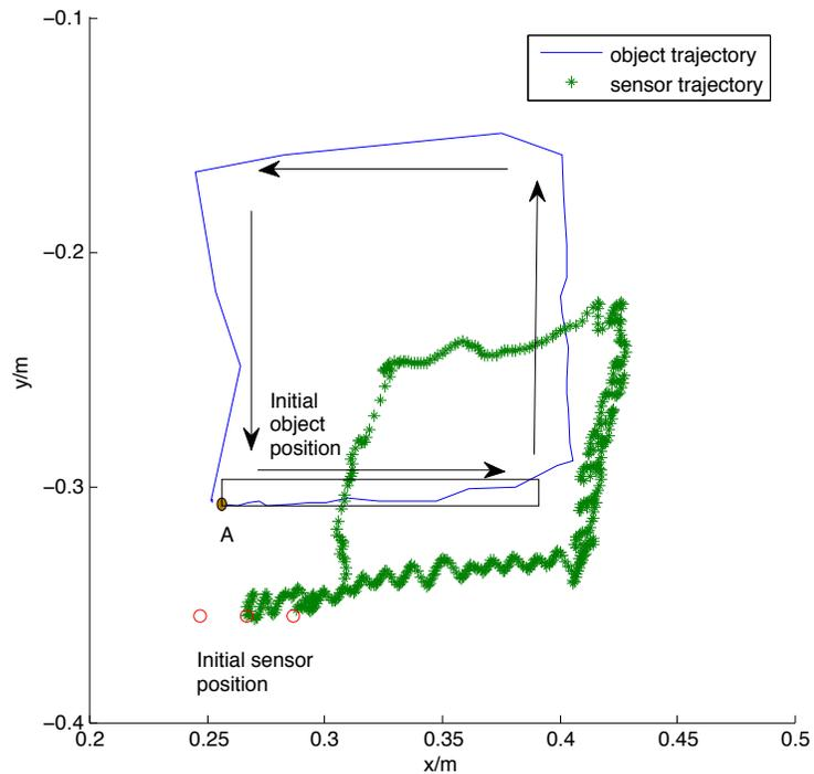
Figure 3.20: Tracking mobile object. The black rectangle is an object. A is a point on the corner of the object. The blue nearly rectangular line is the trajectory of the object. The green stars are the trajectory of sensor 3. The three red circles represent the three sensors. It is with respect to robot base frame.
