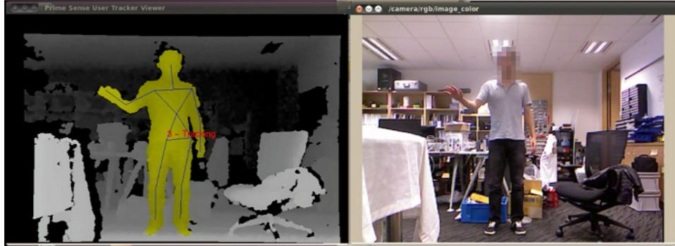
Figure 2.2: Skeleton. The right figure shows the view from Kinect, and the left figure the human skeleton extracted from the sensor data.
