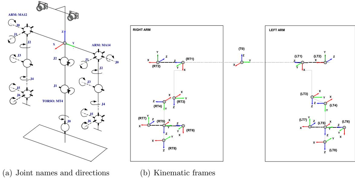
Figure 2.10: MEKA robotics arm joints: (a)the posture shown 0 joint angles, arrows show positive rotation and torque directions; (b) Z axis is the axis of joint rotation [2]
