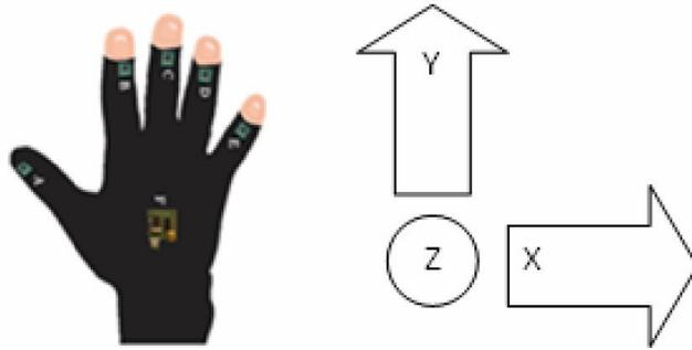
Figure 2.8: acceleglove output signal convention (top view, right hand) [1]
