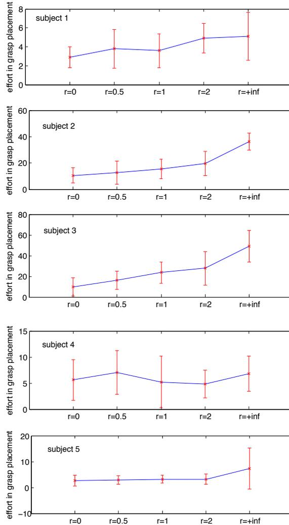
Figure 3.11: Effort in grasp placement for different ratios of teleoperation to assistance. Mean values and standard deviations are shown.
