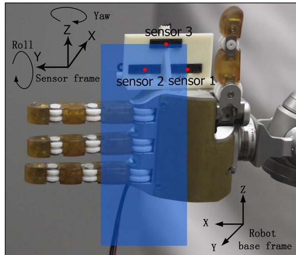
Figure 2.23: Hardware of IR sensors: The red points are the centers of sensor, and two edges of objects are supposed to be on the sensor 1 and sensor 3 centers as the blue rectangular.
