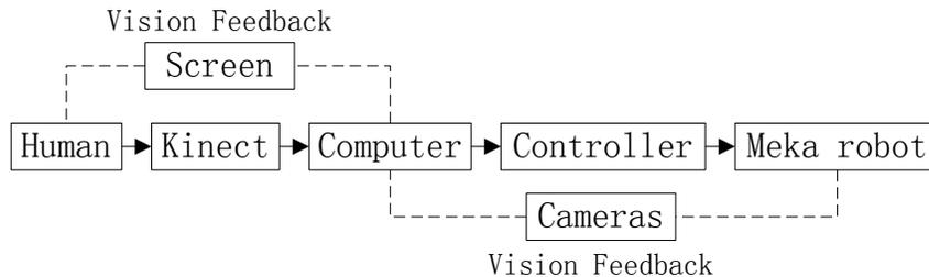
Figure 2.1: Overview of the proposed teleoperation structure
