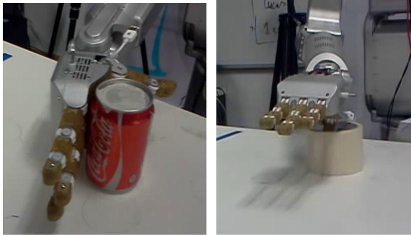
Figure 3.8: Grasp postures. The left image shows grasping a can. The right image shows grasping a tape.
