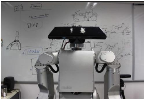
(a) cameras mounted on the robot head
