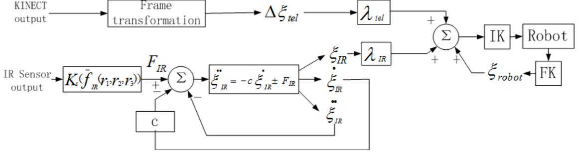
Figure 2.24: Control block diagram. FK and IK denote forward & inverse kinematics maps respectively.
