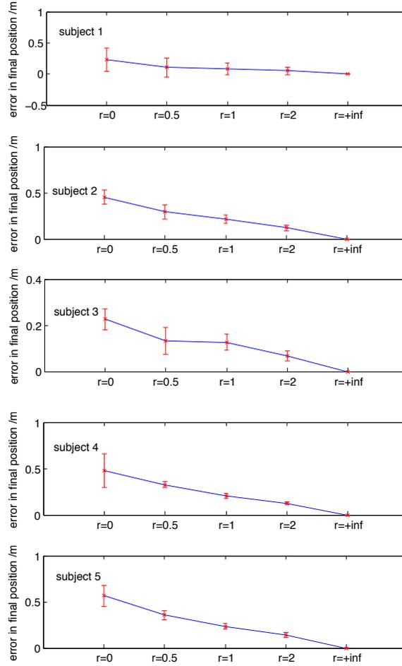
Figure 3.12: Error in final position( $e_f$ ) for different ratios of teleop to assistance. Mean values and standard deviations are shown.
