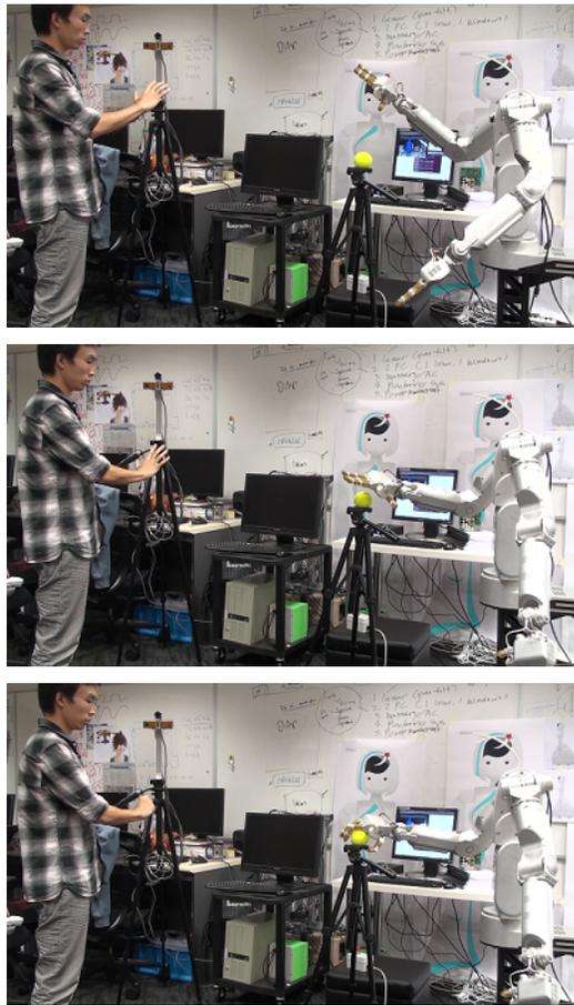
Figure 3.2: Teleoperation with real robot. The first image shows the robot mimics the person to move the arms. The second image shows pre-grasp. The third image shows the robot mimics the person to grasp an object.
