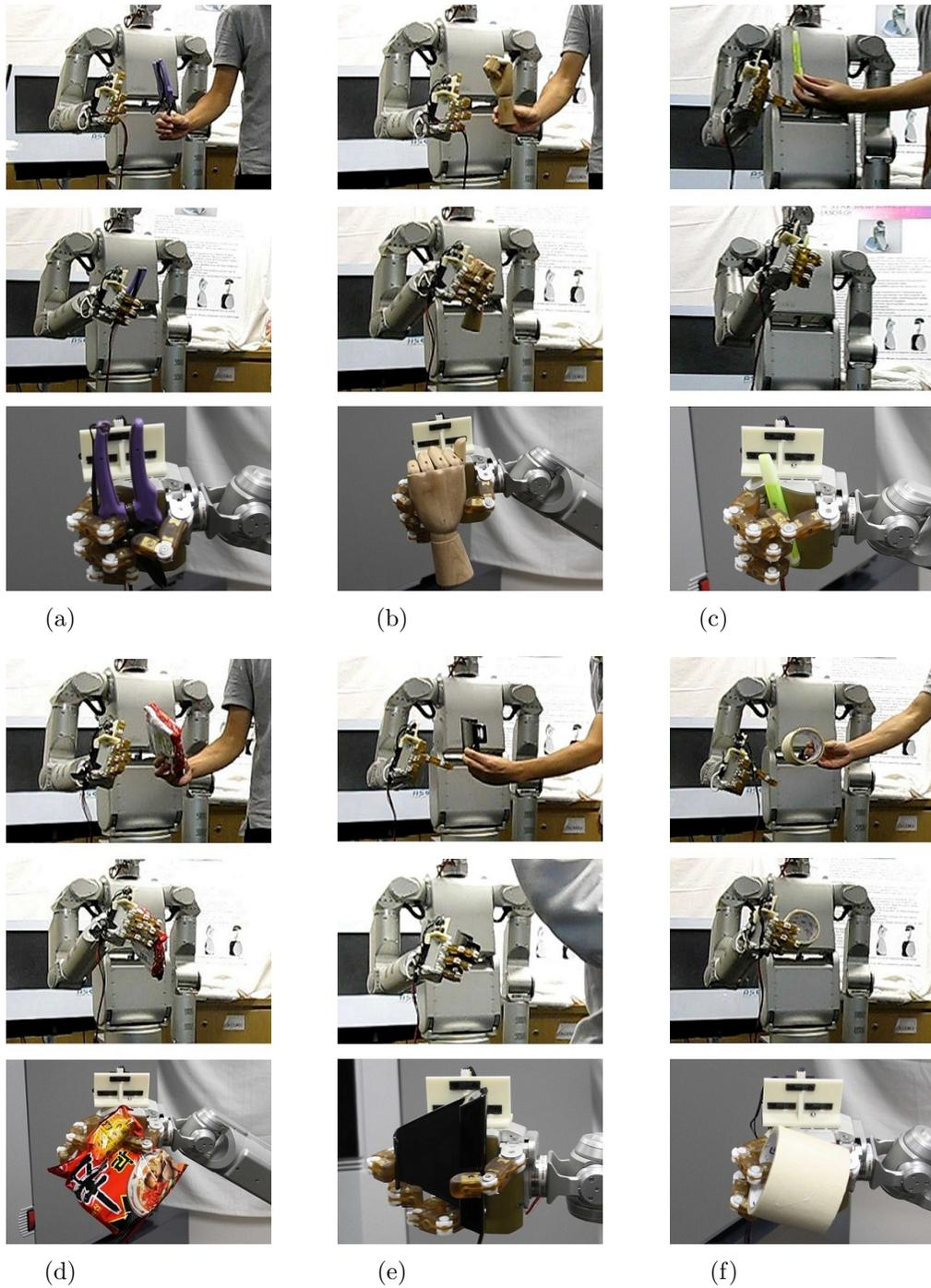
Figure A.2: Grasp experiments: for every object, the top picture shows the initial position of the sensor detecting an object. The middle and the bottom pictures show the final grasp from front view and side view respectively.
