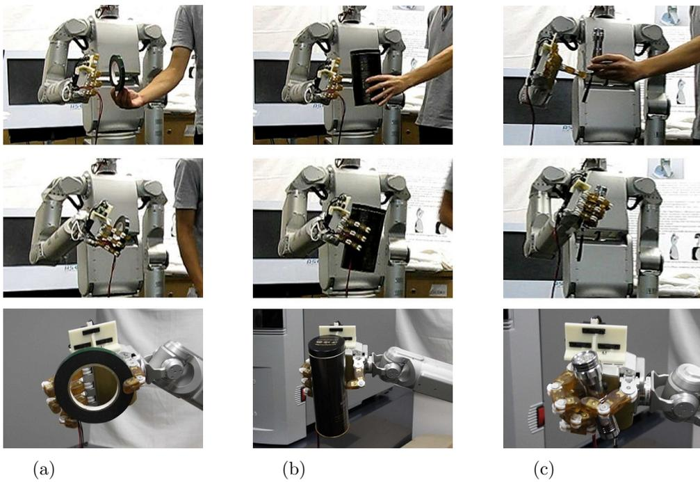
Figure A.3: Grasp experiments: for every object, the top picture shows the initial position of the sensor detecting an object. The middle and the bottom pictures show the final grasp from front view and side view respectively.
