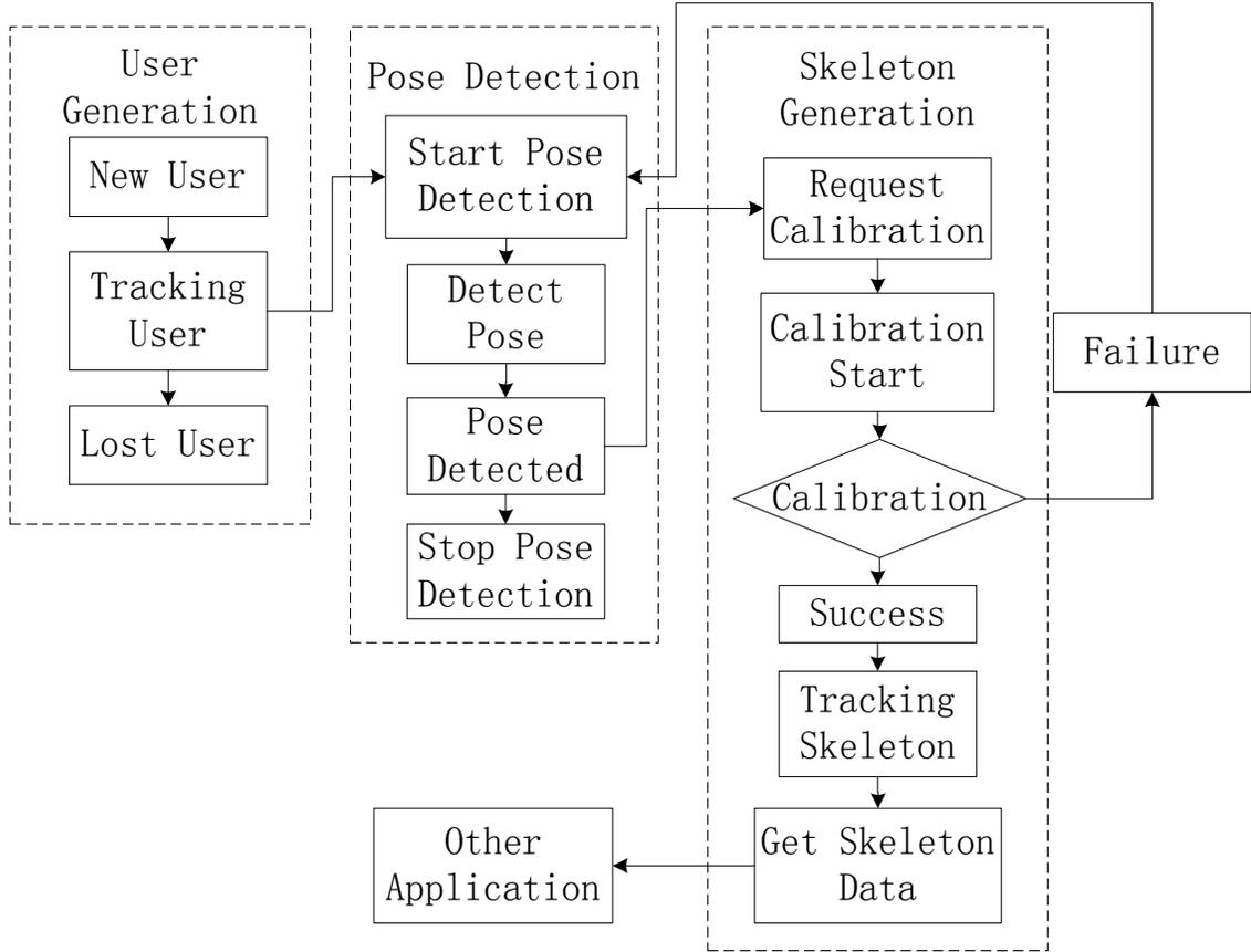
Figure 2.4: Flow chart of detecting joint data
