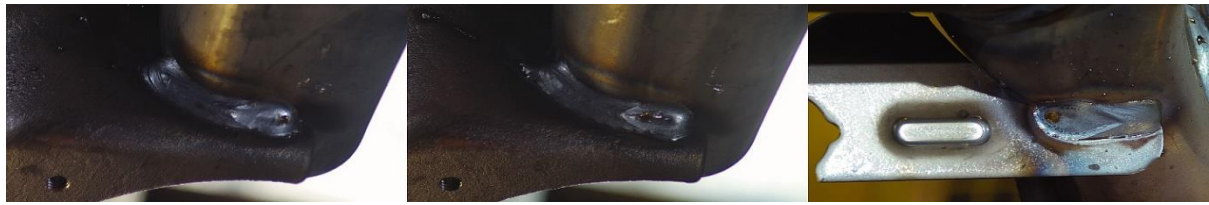
Figure 9: Brightness Anomaly Detection on the Welding Use Case based on PTM monitoring
