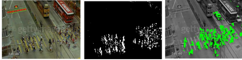
Fig. 5. (a)Sample video frame. (b) Foreground segmentation. (c) Tracking using KLT
