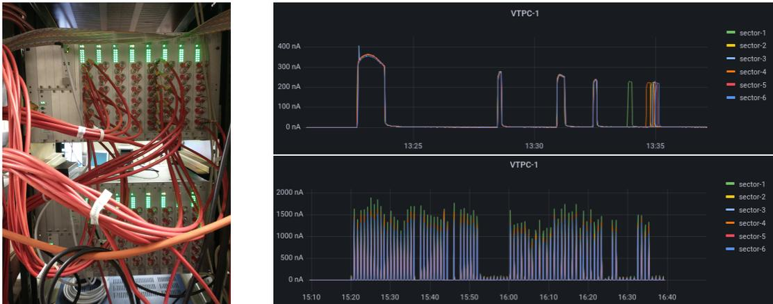
**Figure 2:** *Left:* The photo of the new nanoamp meter crates. *Right top:* The read-out current time-value series in the DCS during ramping individual HV channels, showing negligible cross-leak currents. *Right bottom:* The read-out current time-value series during data taking, showing the in-spill and out-of-spill VTPC-1 anode currents, as an example.
