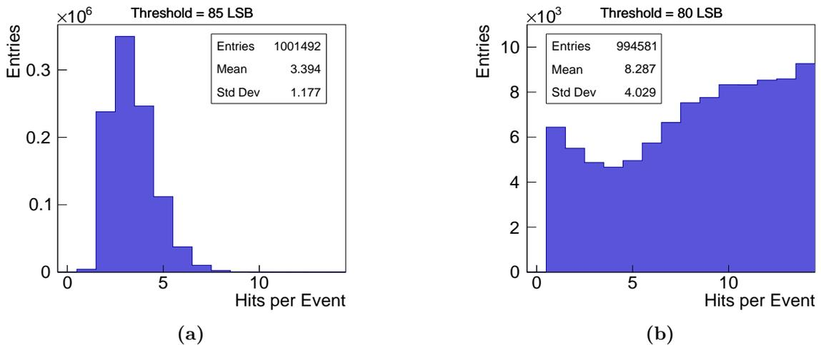
**Figure 10.22.:** Hit multiplicity per event for two different thresholds in a NoBias sensor. At a threshold of 85 LSB (a) an average hit multiplicity of 3.4 is found in the data. Lowering the threshold to 80 LSB introduces a lot of noise hits, which increases the hit multiplicity in the Single MaPSA assembly to 8.3.
