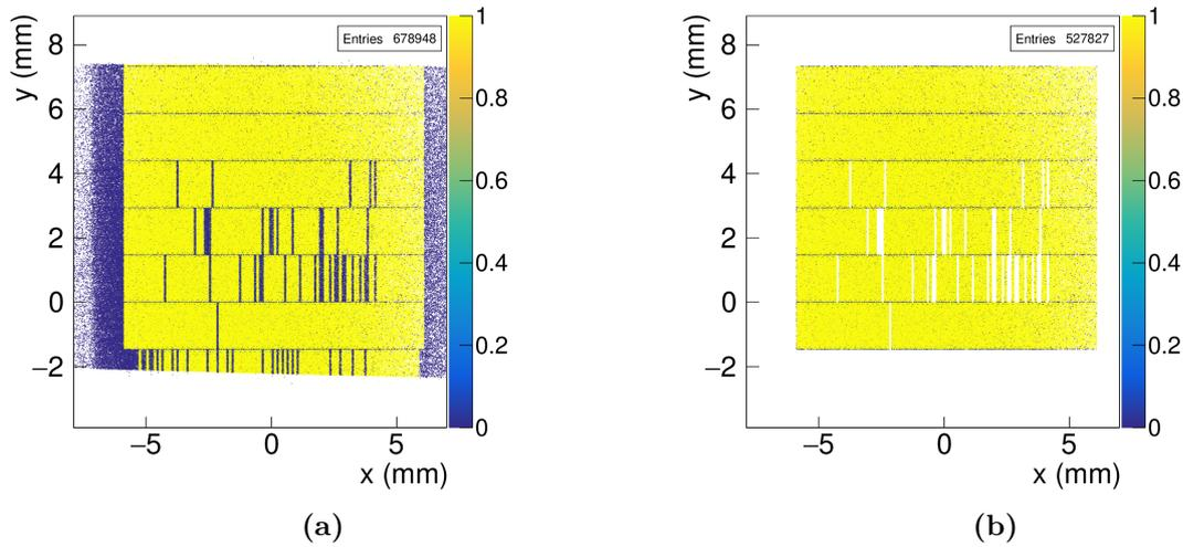
**Figure 10.15.:** Unmasked (a) and masked (b) efficiency map of a Single MaPSA at the CERN beam test. Many unbonded pixels and the passive area around the pixel matrix are responsible for a reduced global efficiency of the assembly. By properly masking these areas, the global efficiency is increased significantly.
