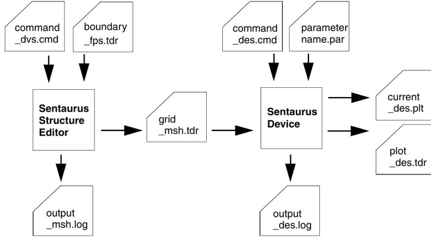
**Figure 7.1.:** The Sentaurus TCAD workflow. The Sentaurus Device Editor takes the geometry files and generates the corresponding mesh file for the device simulation. The mesh file is passed to the Sentaurus Device simulator, which again loads certain script files with all necessary physics models and the desired simulation instructions. The simulation results are stored in two different output files that serve as input for the final analysis [Syn18a].
