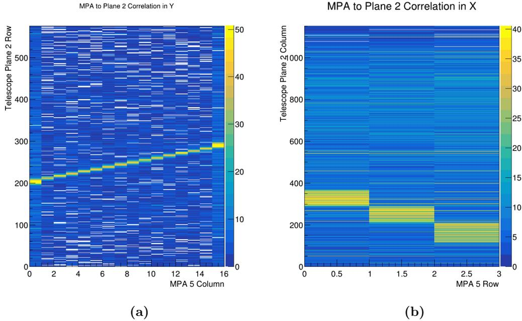
**Figure 6.10.:** Correlation between MPA 5 and the last upstream plane (Plane 2) of the telescope. The two systems are mounted at an angle of  $90^\circ$  towards each other, leading to correlation between MPA columns and telescope rows and vice versa. Correlated hits are clearly recognizable as bin entries along a straight line (yellow) through the plot.
