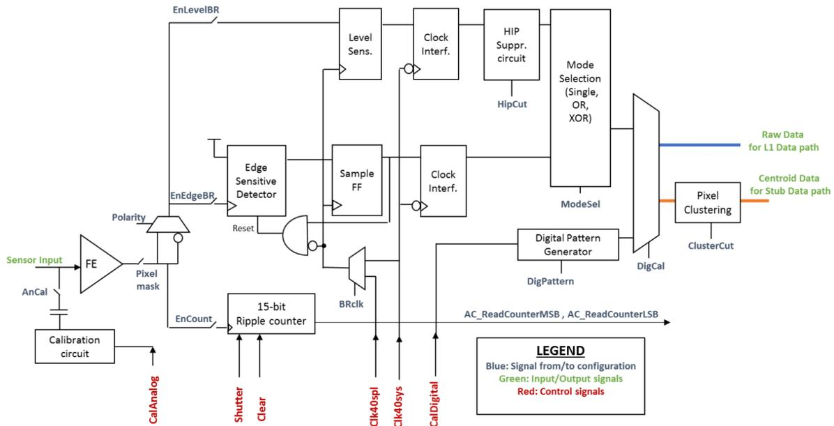
**Figure 10.2.:** The MPA binary readout schematic. The signal of the analog front-end (FE) can be processed by three different acquisition circuits: the edge and level sensitive synchronous readout paths (EnLevelBR and EnEdgeBR) as well as the asynchronous ripple counter (EnCount). The input signal is either provided by the attached sensor or the calibration circuit [Cer+17].
