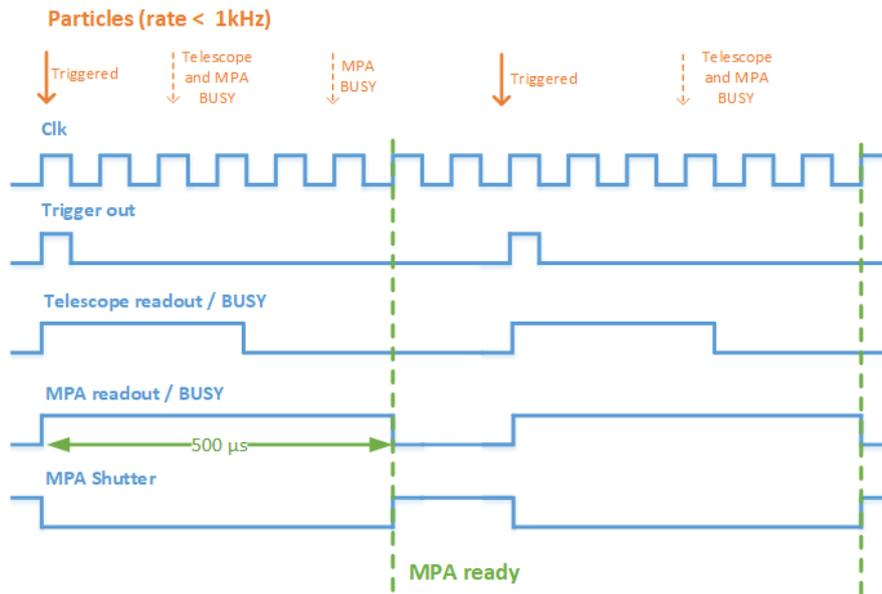
**Figure 6.7.:** Trigger logic at the MaPSA light test beam. When a particle arrives (orange arrow) and all busy lines are set to low, the TLU issues a trigger and sends it to the connected systems. As soon as the trigger is registered by the MaPSA readout, the MPA-Light closes its shutter and simultaneously raises the busy line and starts its readout. After the readout has been completed, the shutter is opened again and the busy line is released.
