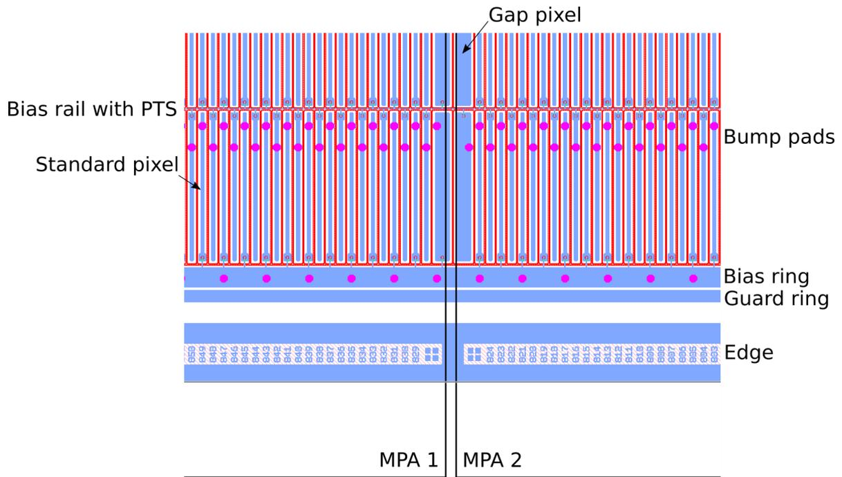
**Figure 8.4.:** One section of the PS-p pixel matrix. Gap pixels with a pitch of  $200\ \mu\text{m}$  below the edge of each MPA cover the additional space between two neighboring readout chips. In total, 31 bias rails run in between the pixel rows, connecting the individual PTS with the bias ring.
