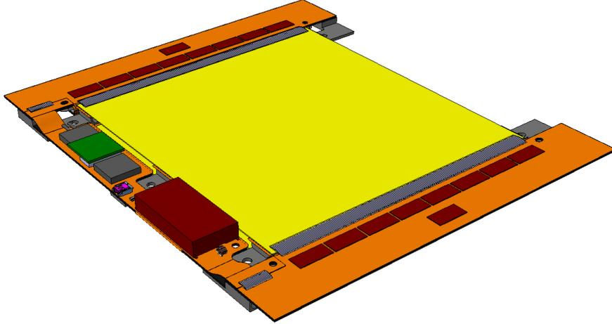
**Figure 3.5.:** Drawings of a 2S module with 4 mm spacing between the sensors. Every strip of the segmented sensors (yellow) is bonded to one channel of one out of 16 CMS Binary Chips (CBCs) that are placed on two front-end hybrids alongside the concentrator chip (CIC) (brown rectangles). Both front-end hybrids are connected to the service hybrid that provides all necessary voltage regulators and the optical transceiver stage to send (and receive) data to the external system [CER18b].
