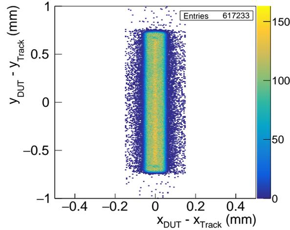
**Figure 10.13.:** Two-dimensional residual distribution of a Single MaPSA. Combining the  $x$  and  $y$  residual distribution reveals the superposition of all pixel cells of the Single MaPSA that are covered by the telescope. The alternating PTS are indicated as small dots with fewer entries at the top and bottom of the pixel cell.
