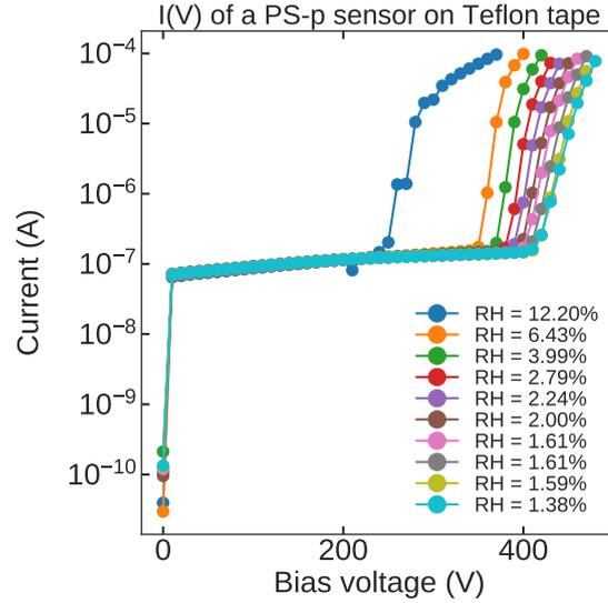
**Figure 9.7.:** Humidity dependence of the breakdown voltage of the full-size PS-p. Although the overall leakage currents remains the same for all measurements, the breakdown voltage is shifted to higher bias voltages with decreasing humidity in the probe station enclosure.
