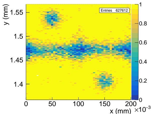
**Figure 10.17.:** Zoomed modulo efficiency map of a Single MaPSA equipped with a Standard sensor. The two bias dots of the PTS are clearly visible. The area between the two pixel rows is severely affected by the efficiency loss. Particularly low efficiencies are encountered in the corner between four pixel cells, which is most likely caused by the charge sharing effect.
