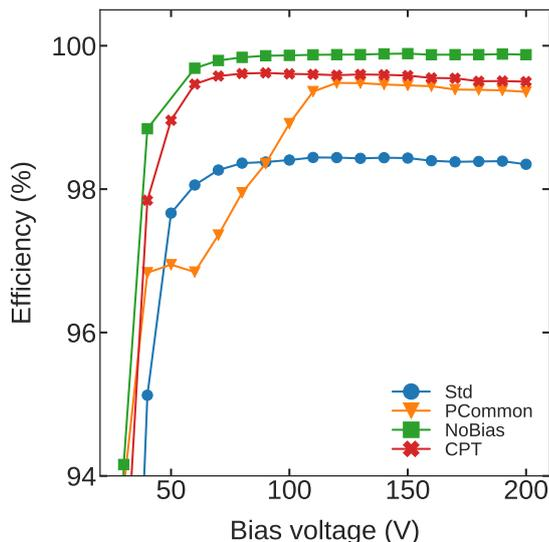
**Figure 10.19.:** Efficiency of four different PS-p single sensors at various bias voltages. All but the PCommon sensor show a very similar turn-on behavior and a minimum operation voltage around 70 V to 90 V. The PCommon sensor, however, shows an unexpected behavior between 50 V and 100 V.
