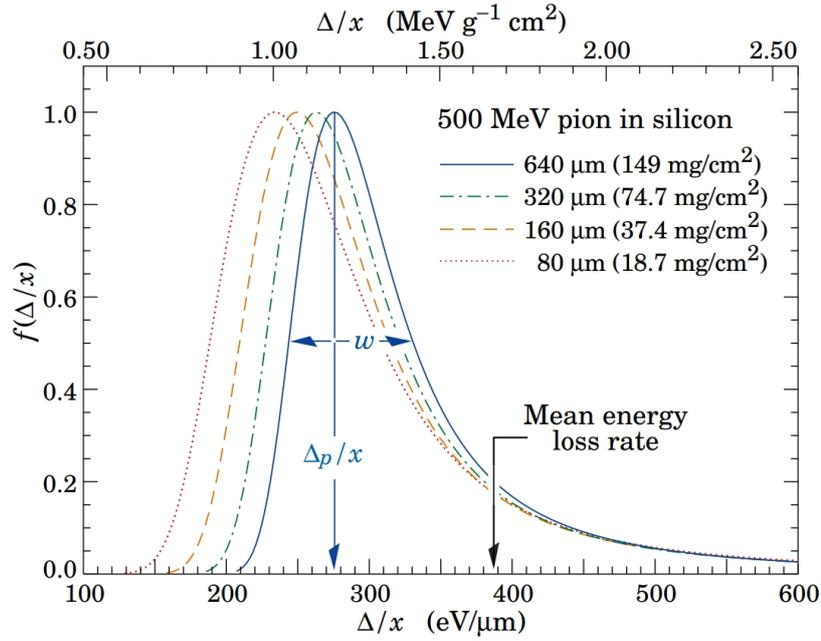
**Figure 4.5.:** Normalized energy deposition per  $\mu\text{m}$  of a 500 MeV muon in silicon with various thicknesses. The energy deposition follows the Landau distribution with an asymmetry tail towards higher energies [Par18].
