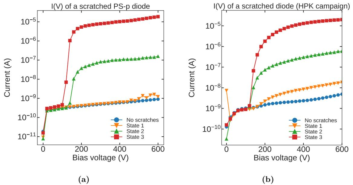
**Figure 9.3.:** Consecutive I(V) measurements of two scratched FZ200 diodes. Both diodes, one from the PS-p wafers (a) and one included in the HPK campaign (b) initially reveal good I(V) characteristics but show a soft breakdown behavior after scratching the aluminum backside multiple times on the chuck. The states 1 to 3 refer to three consecutive states with an equal degree of scratches between both diodes on the backside.
