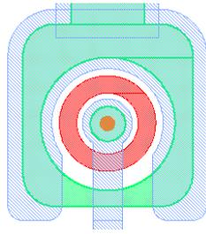
**Figure 5.5.:** A possible implementation of the punch-through structure (PTS). A hole in the pixel implant (green) is used to house the necessary PTS elements. The bias dot (green circle), which acts as seed for the growing depletion region, is conductively connected (orange) to an aluminum rail (blue) which is connected to the global bias grid. An additional p-stop ring (red) isolates the pixel implant and prevents the pixels from short circuits to the bias dot.
