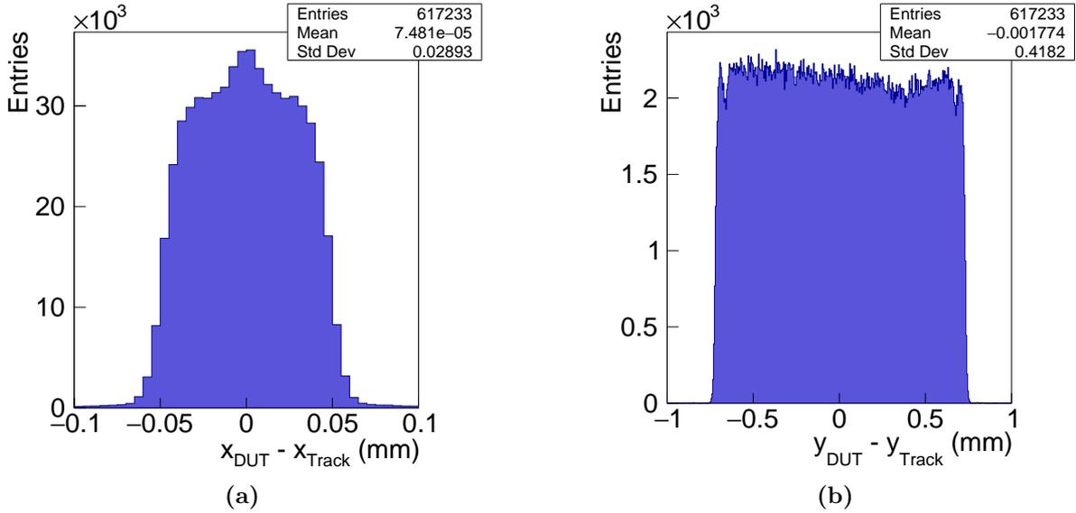
**Figure 10.12.:** Residuals of a Single MaPSA equipped with a Standard sensor. The distributions yield an  $x$  and  $y$  resolution of  $28.9 \mu\text{m}$  (a) and  $418.2 \mu\text{m}$  (b), respectively. Both values are in good agreement with the expected binary resolution of a Single MaPSA. The two noticeable dips in the residual distribution along the long side of the pixels (b) are caused by the inefficient punch-through structures of the Standard layout.
