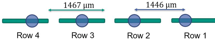
**Figure 8.3.:** Shifting bump bond pads on the PS-p. Since the pixel pitch is different to the pitch of the bump bond pads on the readout chip, the latter have to be shifted within the pixel cells across the pixel rows.
