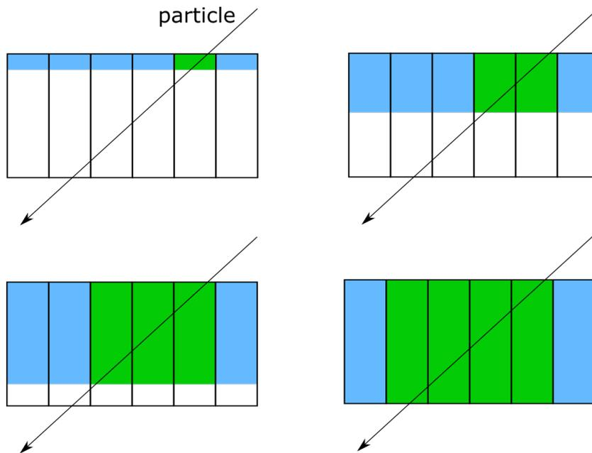
**Figure 10.23.:** Sketch of a cluster size measurement at high incidence angle. With increasing bias voltage, the sensitive space charge region (blue) grows further to the backside, causing more pixels to be activated (green) by particles with a high angle of incidence to the sensor.
