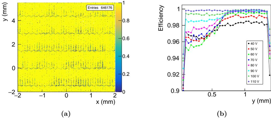
**Figure 10.20.:** Efficiency of the PCommon sensor at bias voltages below 100 V. The efficiency map (a) reveals that all pixels show severe inefficiencies in the lower half of the pixel cell. By increasing the bias voltage (b), the efficiency first decreases before it fully recovers at a bias voltage of 110 V.
