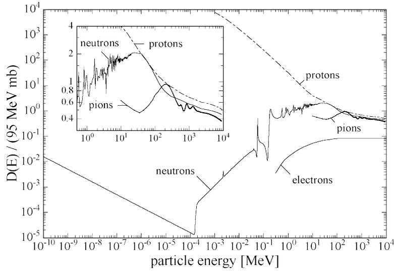
**Figure 4.8.:** Displacement damage functions  $D(E)$  normalized to 95 MeV mb for neutrons, protons, pions and electrons over an energy range of  $10^{-10}$  MeV to  $10^4$  MeV [Mol99].
