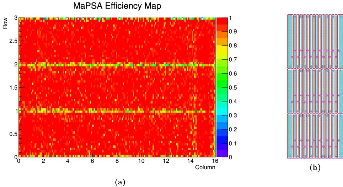
**Figure 6.12.:** Efficiency map of the PS-p light read out by one of the two bump bonded MPAs (a). Almost all parts of the observed area are fully efficient. Only in the region between the individual pixel rows the efficiency can drop to about 60 % which can be traced back to the aluminum bias rails that are running across the pixel matrix (b).
