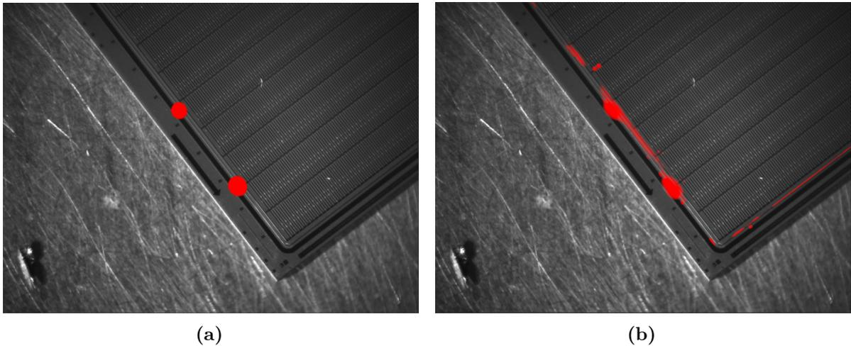
**Figure 9.13.:** Infrared imaging of a PS-p single sensor at different humidities. The sensor is operated at 300 V and above its breakdown voltage. Locations with high current densities are marked in red. At a relative humidity around 14 % only the guard and bias ring show two local breakdowns (a). At an increased humidity of approximately 35 % in the probe station enclosure, more areas along the periphery as well as parts in the pixel matrix get affected (b).
