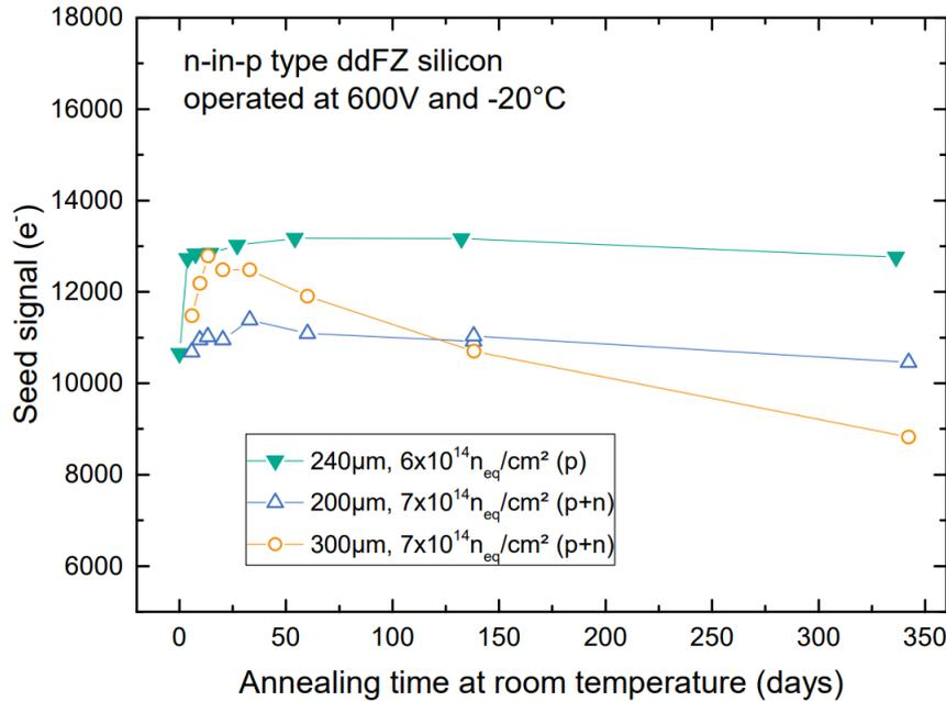
**Figure 5.4.:** Annealing behavior of sensors with three different thicknesses after an irradiation to  $6 \times 10^{14} n_{eq}/cm^2$  and  $7 \times 10^{14} n_{eq}/cm^2$ . The material with an active thickness of  $300 \mu m$  shows a pronounced annealing behavior with significant reverse annealing after approximately 20 days at room temperature. Seed signals which are generated in thinner material on the other hand stay more or less constant over long period of time [CMS18].
