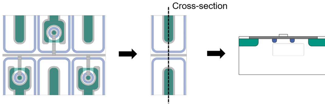
**Figure 7.2.:** Generation of the device geometry for the simulation. The initial PS-p light geometry is simplified by omitting the punch-through structure and only considering two adjoining pixel cells. In order to reduce the mesh size and computing time, only a two dimensional simulation is performed.
