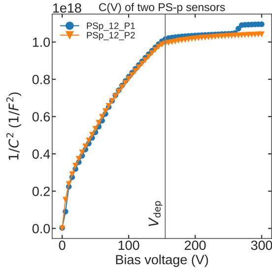
**Figure 9.8.:**  $C(V)$  characteristics of the full-size PS-p. The noticeable kink at about 150 V marks the point of the full-depletion voltage  $V_{\text{dep}}$ . The second step, seen on one of the two full-size sensors, indicates a sudden and unexpected decrease in capacitance.
