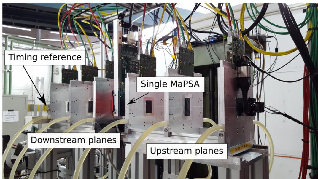
**Figure 10.10.:** Single MaPSA test beam setup at DESY. The Single MaPSA (DUT) is mounted on two movable and one rotational stage between the three upstream and three downstream planes of the DATURA telescope. The CMS pixel timing reference is placed behind the last downstream plane.
