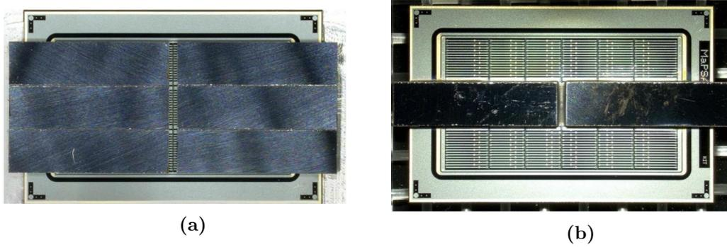
**Figure 5.17.:** Two MaPSA light assemblies. In order to read out all macro-pixels, the PS-p light is supposed to be equipped with six MPA-Lights (a). However, due to unexpected dicing issues, most assemblies produced at KIT only contain two readout chips (b).
