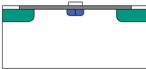
**Figure 7.9.:** Schematic of the common p-stop design. The individual p-stop rings are merged together, forming the desired common p-stop configuration (blue). In this approach, the bias rail (gray) on top of the oxide (dark gray) is effectively shielded by the p-stop, preventing the electrons from accumulating below the silicon dioxide and therefore reducing the charge collection efficiency.
