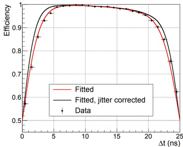
**Figure 6.6.:** The MPA-light hit efficiency as a function of the phase difference between the particle arrival and the 40 MHz clock of the MPA-Light. The red curve represents the fit to the data points while the black curve shows the jitter corrected efficiency distribution. The timing jitter is introduced by the difference in frequency of the beam clock and MPA-Light clock [CMS18].
