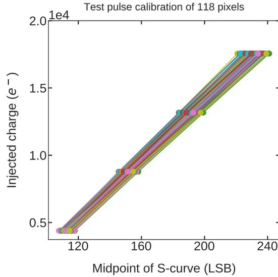
**Figure 10.31.:** Test pulse calibration of 118 pixels on one exemplary assembly. All pixels show a linear response behavior. The average slope of all 118 pixels is  $(107 \pm 2) e^-/\text{LSB}$ .
