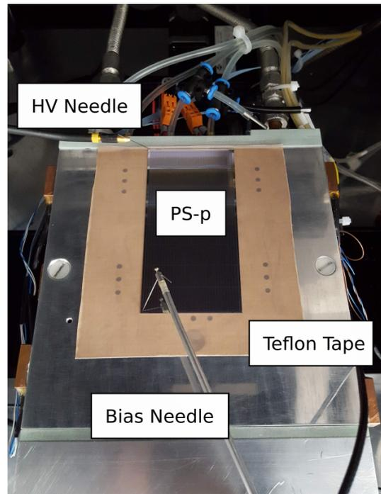
**Figure 9.5.:** Front-side biasing arrangement for the full-size PS-p. In order to protect the sensor backside, the full-size PS-p is placed on a protective Teflon tape and is biased through the sensor edge, using the frontside biasing approach.
