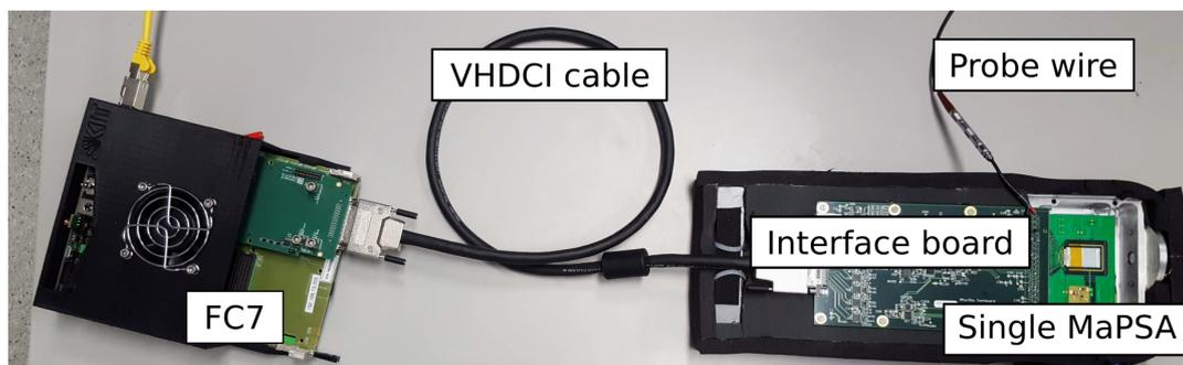
**Figure 10.6.:** The Single MaPSA test setup. The Single MaPSA on its carrier board is plugged into the PCI-e connector on the interface board, which provides all necessary voltage levels to operate the MPA. The interface board is connected to the FC7, which is used to control and read out the MPA. The FC7 uses an Ethernet connection to send and receive data from the connected readout PC.
