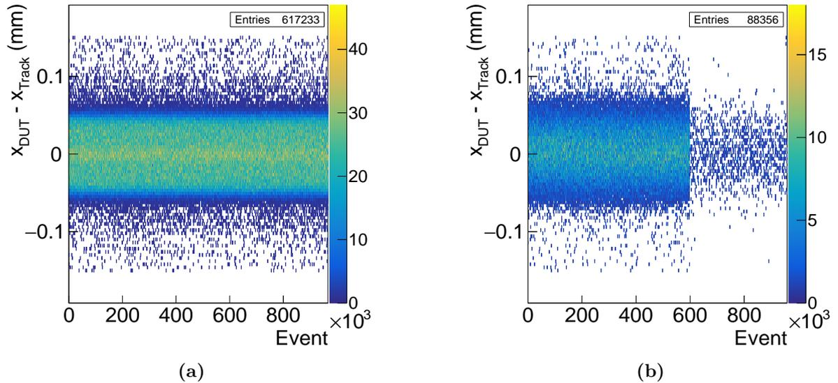
**Figure 10.14.:** Residual in  $x$  over the event number. Figure (a) shows perfect synchronization without any irregularities throughout the entire run. In figure (b), the residual distribution changes immediately as soon as synchronization is lost after about 600 000 events.
