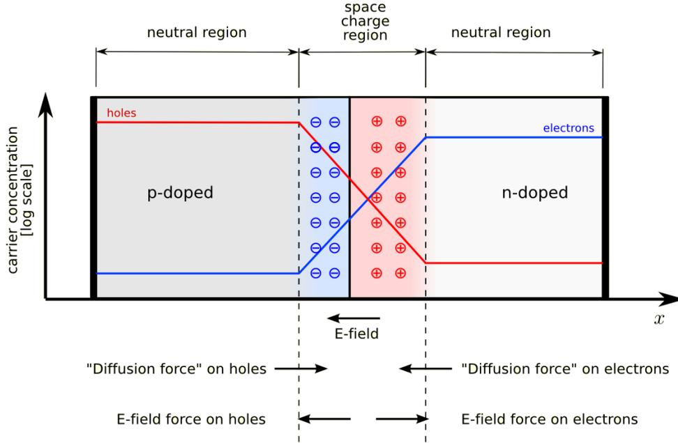
**Figure 4.3.:**  $pn$ -junction in equilibrium. The diffusion of majority charge carriers is compensated by an electric field that is generated by the recombination process of electrons and holes in the space charge region (SCR). The forces caused by the diffusion and the electric field are shown below the  $pn$ -junction. The corresponding electron and hole concentration are marked in red and blue, respectively [The07].
