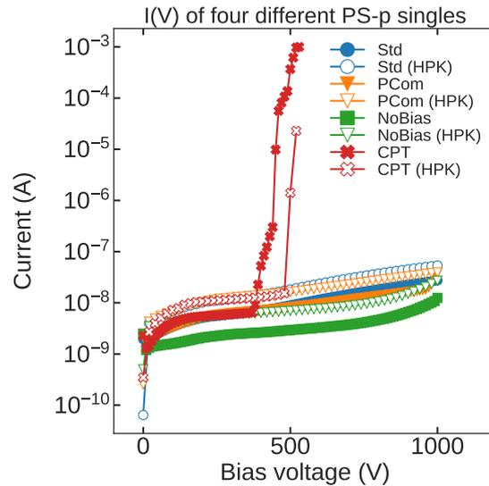
**Figure 9.10.:**  $I(V)$  measurements of the PS-p single sensors. Only the quite aggressive common punch-through layout (CPT) shows an early breakdown at around 400 V that has already been observed by Hamamatsu. The NoBias design shows a lower leakage current, which is related to the unbiased pixel cells due to the non-existing bias grid.
