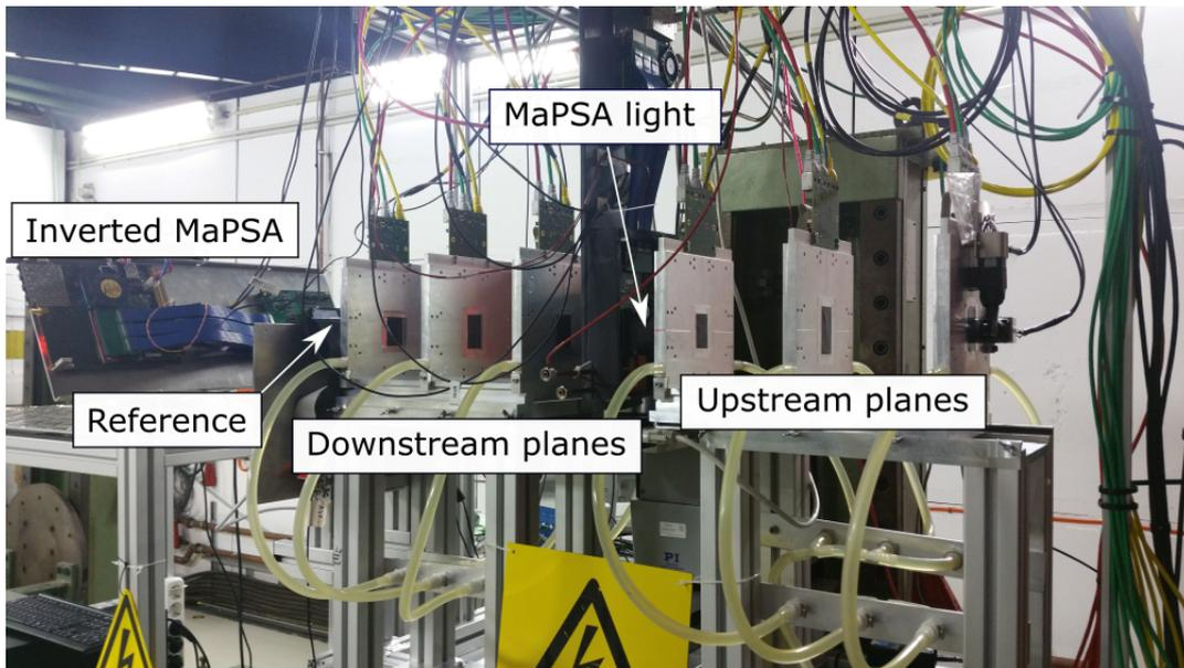
**Figure 6.5.:** The MaPSA light test beam setup. The MaPSA light setup, mounted on a carbon fiber plate, is placed on three movable stages between the telescope arms. The timing reference is mounted on the telescope frame right behind the last plane of the downstream arm. The inverted MaPSA setup is placed on a separate table behind the telescope.
