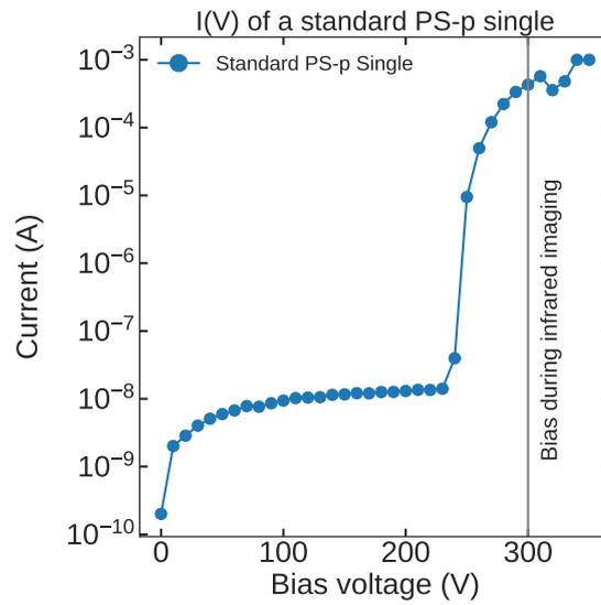
**Figure 9.12.:**  $I(V)$  of a Standard PS-p single used for the infrared imaging. The sensor shows a noticeable breakdown at bias voltages around 250 V. During the infrared image analysis the sensor has been operated at 300 V (gray vertical line).
