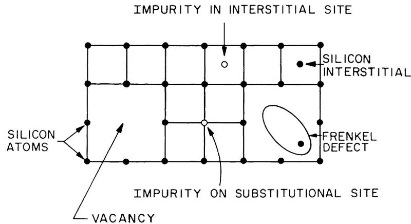
**Figure 4.7.:** Possible bulk defects in a crystal lattice. Atoms can be knocked out of their lattice sites and thus create *vacancies* at their former positions. The released atom can then occupy one of the surrounding *interstitial* sites and create a double defect called *Frenkel pair* [Lut07].
