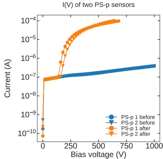
**Figure 9.2.:** Two consecutive I(V) measurements of two full-size PS-p sensor before and after dicing. During the first measurements (blue) no breakdowns were observed. However, if the same two sensors are measured again the day after storing it in its original packaging, the soft breakdown reappears.
