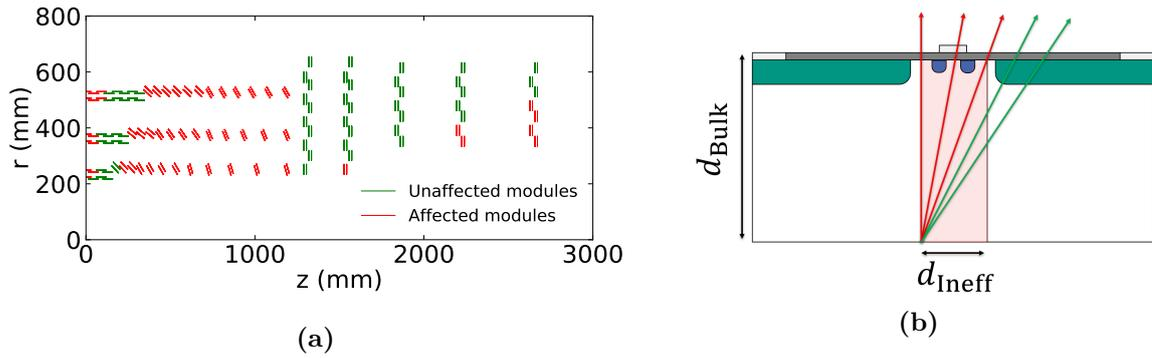
**Figure 10.32.:** PS modules in one quarter of the CMS Tracker that are affected (a, red) or unaffected (a, green) by an efficiency loss below the bias rail. A module is defined as affected, if a particle can pass the sensor solely within the inefficient area (b, red arrows) below the bias rail. If the particles always pass the efficient area of the sensor, the module is regarded as unaffected (b, green arrow). About 46 % of the PS modules are affected by an efficiency loss.
