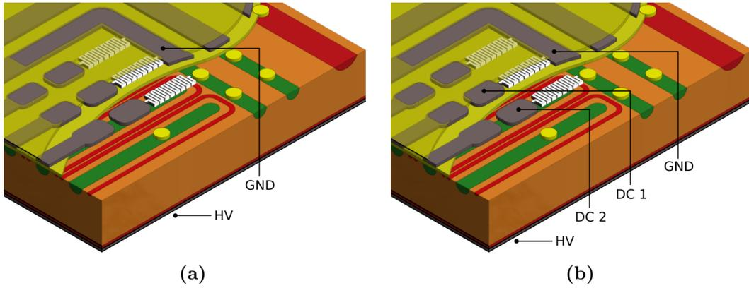
**Figure 5.10.:** Needle configurations for PS-p measurements. For  $I(V)$  and  $C(V)$  (a) measurements only one needle has to be placed onto the bias ring and set to ground potential, while the backside of the sensor is set to high voltage. For pixel and inter-pixel measurements (b) up to two additional needles have to be placed onto two adjoining DC (bump bond) pads.
