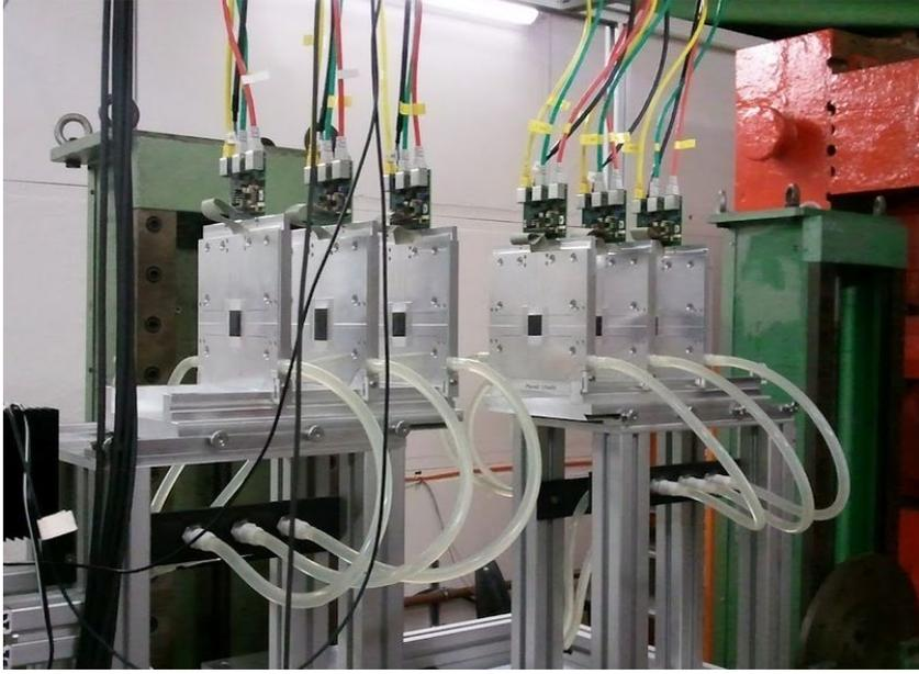
**Figure 6.2.:** The DATURA telescope at the DESY test beam. The telescope consists of two arms with three MIMOSA 26 sensor planes each. The three planes closer to the accelerator (right side of the picture) are called upstream planes and the three remaining ones are called downstream planes, respectively [Deu18].
