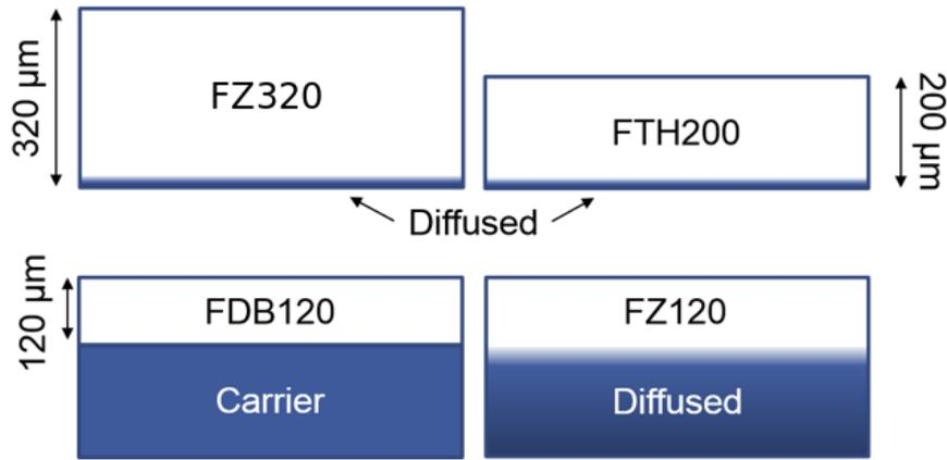
**Figure 5.1.:** Schematics of silicon substrates of various physical and active thickness. The base material is a  $320\ \mu\text{m}$  thick silicon wafer with a thin backside implant. To reduce the the active thickness, the wafer can either be thinned down (TH) directly or after it is bonded onto a carrier wafer. A third option is a deep diffused backside implant which is offered exclusively by Hamamatsu Photonics K.K.
