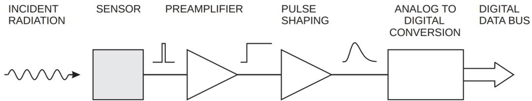
**Figure 5.14.:** Signal processing of a readout chip. The short pulse that is generated inside the sensor is passed to the preamplifier which integrates and amplifies the incoming signal and passes it to the pulse shaping circuit. There the signal gets differentiated again and smoothed by a low-pass filter. The final shaper output is then digitized and fed into the digital bus of the chip [Spi05].
