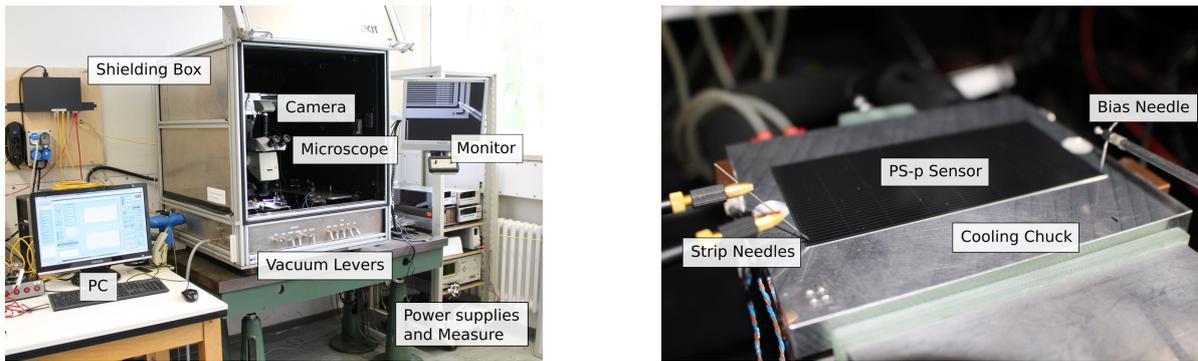
**Figure 5.9.:** Pictures of one out of two probe station setups at ETP. The movable and coolable vacuum chuck is placed in a darkened shielding box which is constantly flushed with dry air. The chuck is surrounded by up to four needles that are used to contact the test pads on the sensors. The power supplies, measuring devices and all other test equipment is controlled by LabVIEW or Python based software package.
