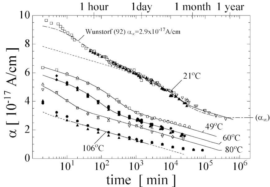
**Figure 4.10.:** Annealing of the current related damage rate  $\alpha$  over time at different temperatures.  $\alpha$  decreases continuously over time at every temperature shown in the plot. The higher the temperature, the lower  $\alpha$  in general [Mol99].
