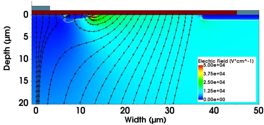
**Figure 7.4.:** Electric field distribution at the frontside of the base design at  $V_{\text{Bias}} = -150$  V. The maximum electric field in the bulk is located at the interface between the p-stop (white line) and the electron accumulation layer below the silicon dioxide. Higher field strengths in the oxide layer are not taken into account.
