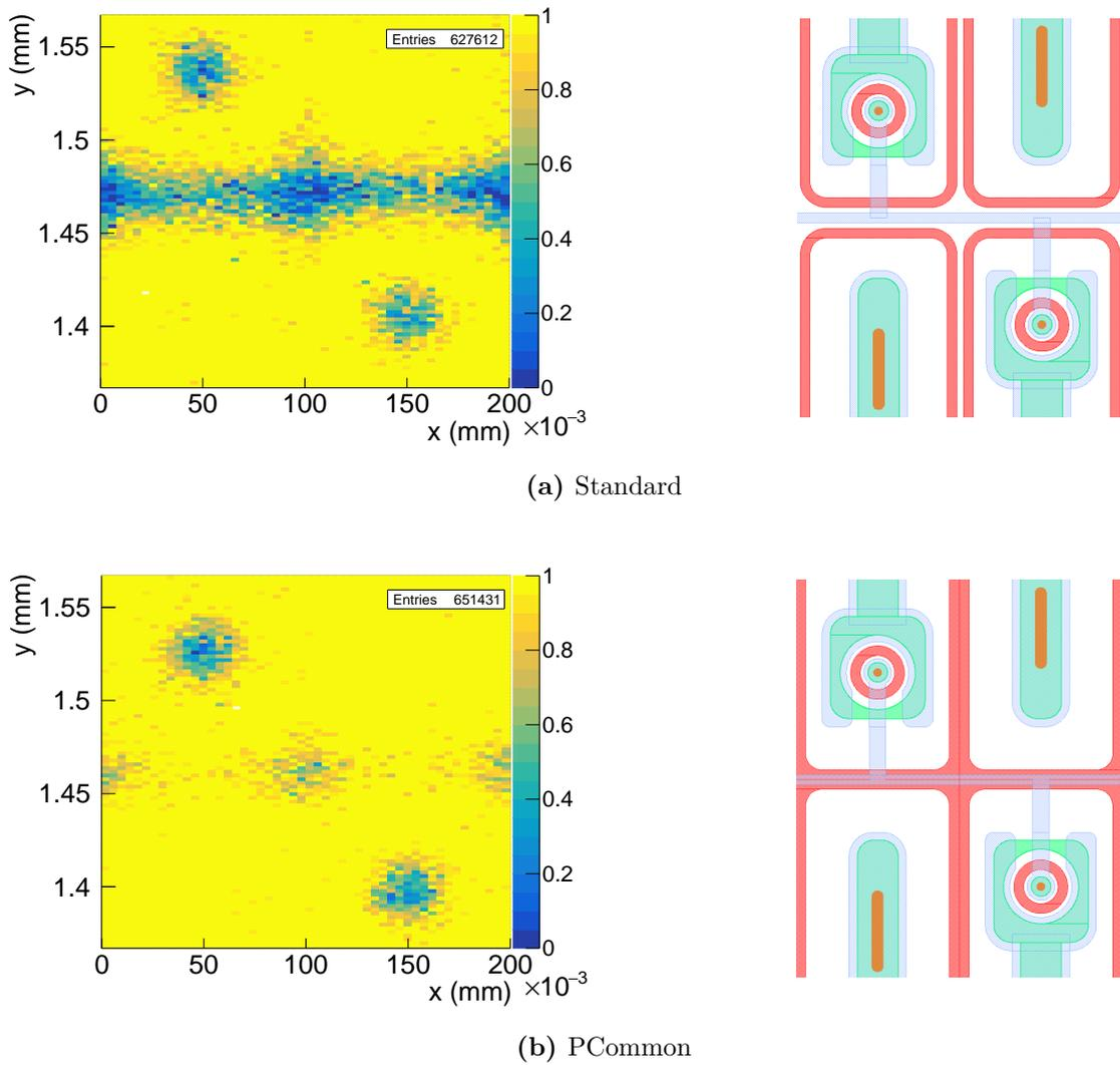
**Figure 10.18.:** Zoomed modulo efficiency maps of two Single MaPSAs equipped with a Standard or PCommon single PS-p sensor at a bias voltage of 200 V and a threshold of 110 LSB. Shielding the bias rail (PCommon) increases the efficiency of the sensor significantly compared to the Standard layout.
