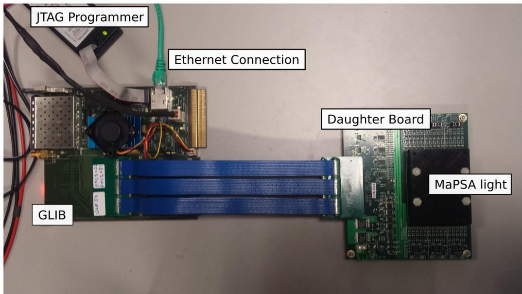
**Figure 5.19.:** The MaPSA light readout system. The MaPSA light carrier board is covered by a 3D-printed enclosure and is connected to the custom made daughter board. A high pin count FMC to FMC cable (blue) connects the daughter board with the FPGA based Gigabyte Link Interface Board (GLIB), which is controlled by a PC through an ordinary Ethernet connection. A JTAG connector provides the necessary interface to upload custom firmware to the board and adapt the FPGA to the user's needs.
