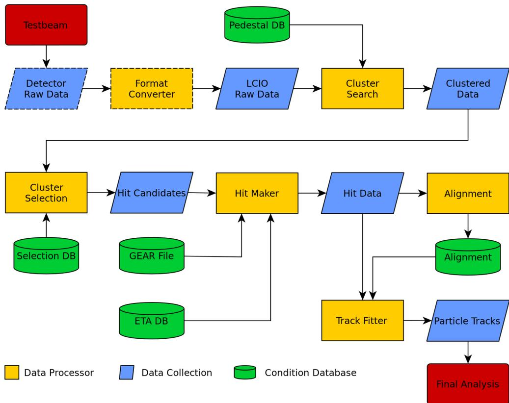
**Figure 6.4.:** The EUTelescope data analysis framework. The raw data from the test beam is converted into the LCIO file format, which is used for every further step in the analysis. A sequence of processors (yellow boxes) uses the data to generate a set of intermediate data collections (blue rhomboids) and databases (green cylinder) which ultimately lead to the reconstructed particle tracks that are used for the final analysis [DES18].
