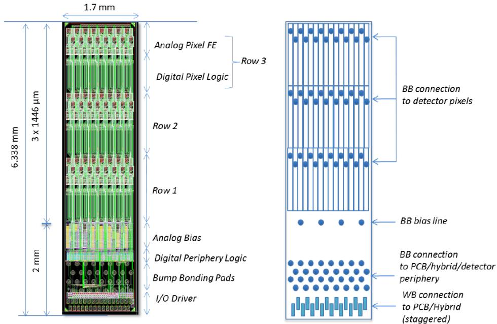
**Figure 5.13.:** Schematics of the MPA-Light. On the left: final design and description of the MPA-Light and its individual sections. On the right: all electrical connections of the chip, including the bump bond pads of the analog front-ends, the ground pads of bias circuit as well as the bump bond and wire bond pads for the external connection [Cer15].
