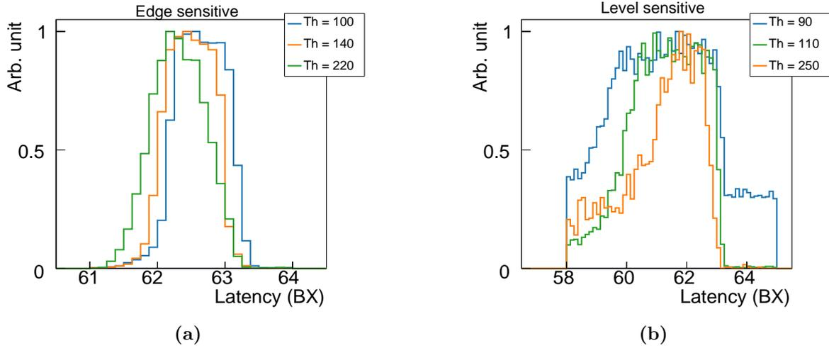
**Figure 10.11.:** Latency scan of a Single MaPSA in edge (a) and level (b) sensitive mode. Due to the time walk of the MPA, increasing the threshold in edge sensitive mode causes the distribution to shift towards lower latency values. In level sensitive mode, increasing the threshold leads to narrower distributions, which are still wider than in edge sensitive mode. The offset at a threshold of 90 LSB is caused by random noise hits that are present for each latency and TDC values.
