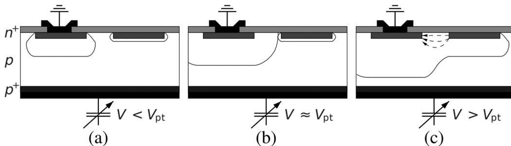
**Figure 5.6.:** An illustration of the punch-through effect (PTE). As soon as the growing depletion region of the connected implant (a) reaches the SCR of the floating implant (b), excess charge carriers are removed and the two depletion regions are getting merged (c) [Ros+06].
