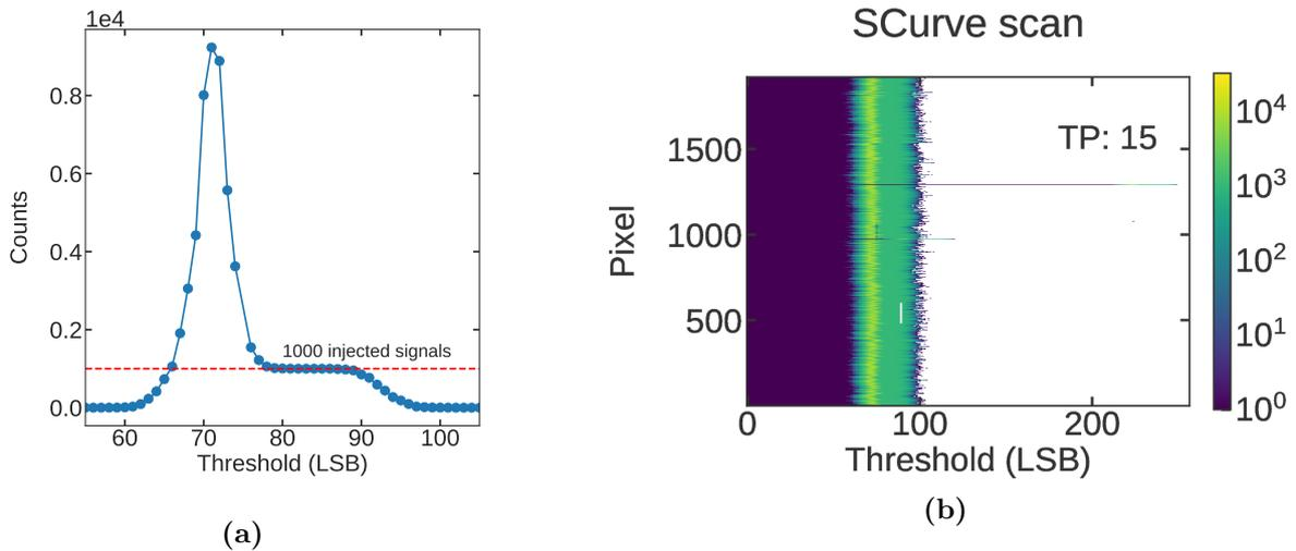
**Figure 10.8.:** Trimming results of a Single MaPSA using 1000 test pulses with an amplitude of 15 LSB at a trim target of 70 LSB. The response behavior of a single channel (a) features the characteristic noise peak at around 70 LSB and the S-curve beginning at 90 LSB. The overall trimming result of the entire chip (b) is very homogeneous and shows only few channels that could not be trimmed properly.
