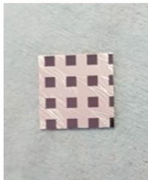
**Figure 9.4.:** Scratches on a diode of the HPK campaign. Even the small number of scratches shown here leads to a soft breakdown of the diode.
