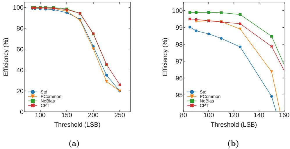
**Figure 10.21.:** Efficiency of four different PS-p single sensors at various thresholds. All four layouts follow the same course in the threshold scan (a). At low thresholds, efficiencies above 99 % can be achieved. With increasing threshold, the efficiency starts to drop to a minimum of about 20 % at a threshold of 250 LSB. By zooming into the region of low thresholds (b) differences in the various sensor designs become visible.
