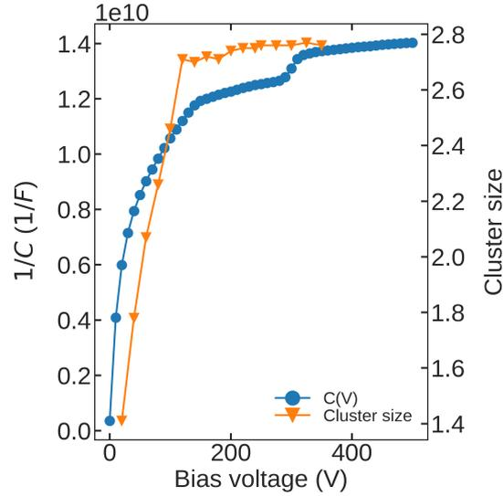
**Figure 10.24.:** Results of a cluster size measurement at an angle of incidence of  $50^\circ$ . At bias voltages below 200 V the course of the cluster size over the bias voltage roughly follows the course of the C(V) measurement in the laboratory. The saturation point at 130 V approximately matches the full-depletion voltage of 140 V. No additional step in the course of the cluster size could be observed.
