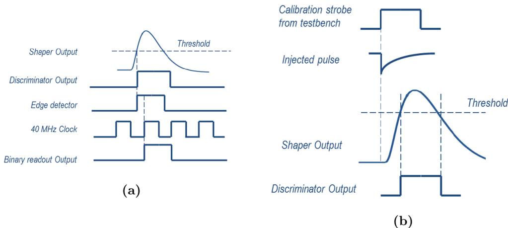
**Figure 5.15.:** The MPA-Light acquisition modes. In synchronous acquisition (a) the discriminator output is passed to an edge detector that generates a signal of exactly one clock cycle which is subsequently sampled by the global 40 MHz clock. The asynchronous acquisition (b) only detects the positive edge of the discriminator output and increases a 16-bit ripple counter that is implemented in every pixel cell [Cer15].
