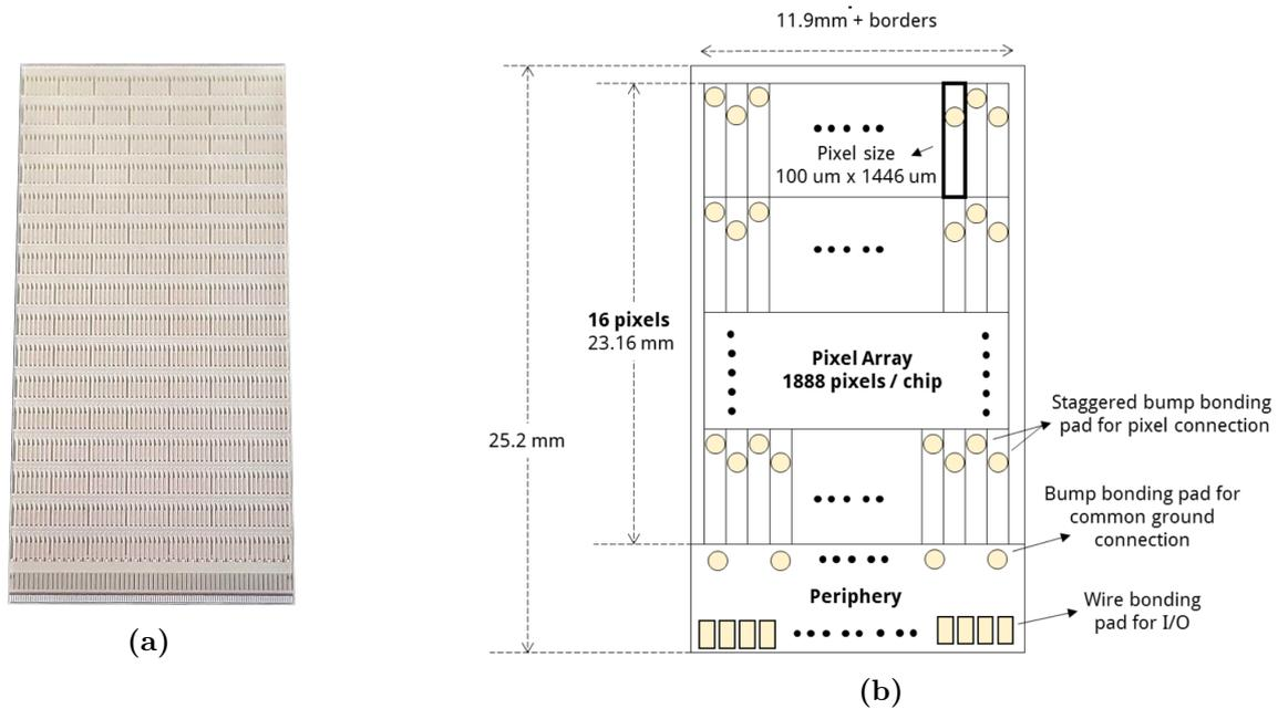
**Figure 10.1.:** Picture of the Macro Pixel ASIC (a) together with a schematic including its dimensions and electrical connections, also known as *floor plan* (b) [Cer+17].
