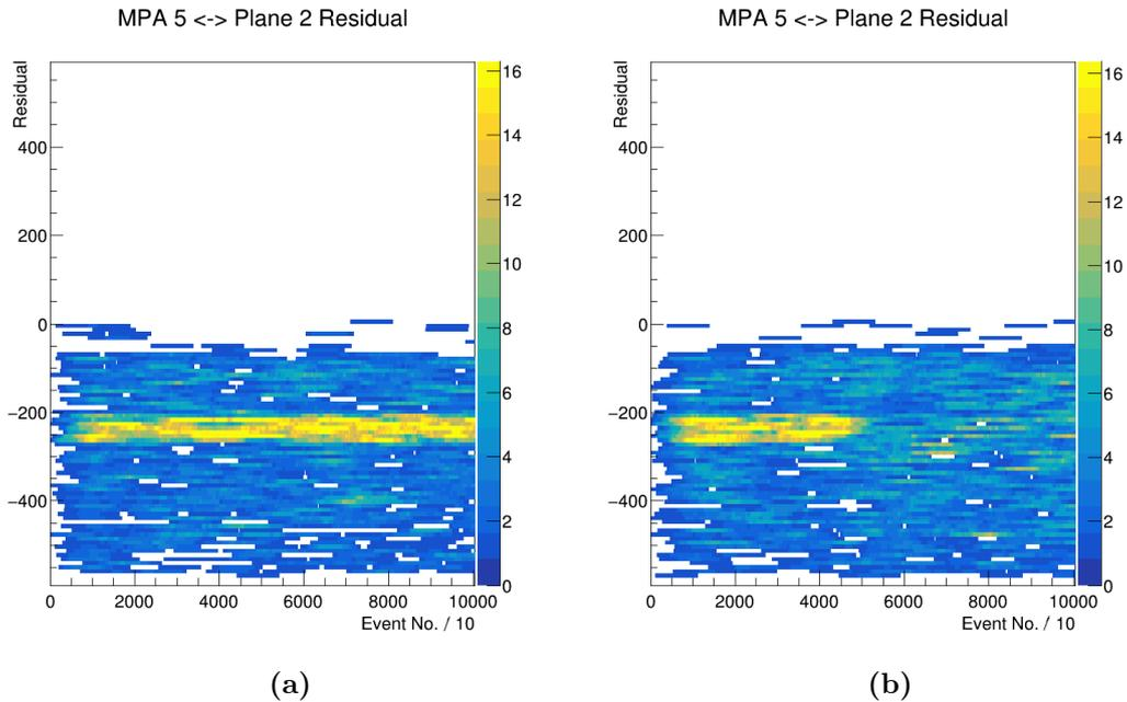
**Figure 6.11.:** Correlation between MPA 5 and the last upstream plane (Plane 2) over the event number. Figure 6.11a shows perfect correlation of the two systems until the end of the run. In figure 6.11b on the other hand a clear sync loss of the data streams is recognizable after approximately 50 000 events.
