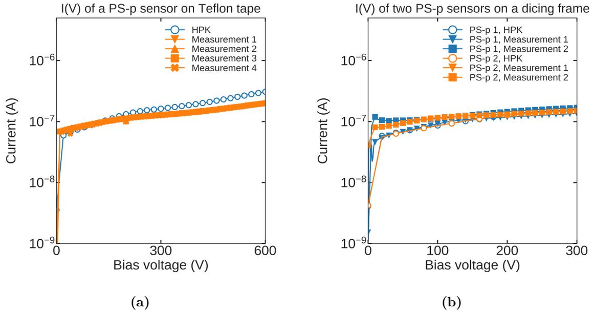
**Figure 9.6.:**  $I(V)$  measurements of the full-size PS-p using frontside biasing. In order to protect the sensor backside, the full-size PS-p is either placed on a protective Teflon tape (a) or is still attached to the dicing frame (b). In both cases, the sensor is biased through its edge, using the frontside biasing approach. In this setup, no soft breakdowns have been observed for multiple consecutive  $I(V)$  measurements of the full-size sensor.
