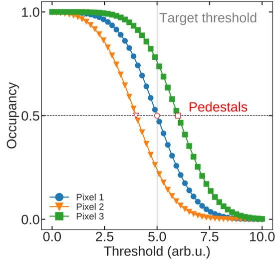
**Figure 10.7.:** Illustration of three exemplary S-curves with different pedestals. The pedestals of two of them do not match the target threshold of 5 arb.u. and thus need to be trimmed.
