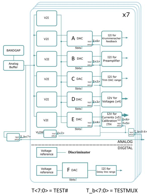
**Figure 10.4.:** Illustration of the MPA bias structure. The bias structure is split into seven individual bias blocks that can be calibrated independently. Each bias block includes six digital to analog converters (DACs) that are used to adjust the output currents and voltages for the analog front-end [Cer+17].
