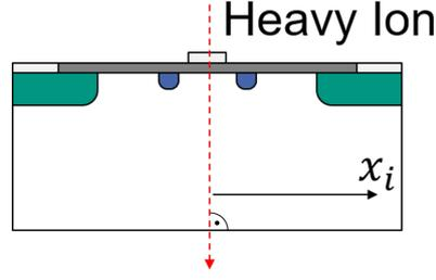
**Figure 7.7.:** Schematic of a heavy ion simulation of the standard geometry. The charged particle penetrates the sensor at the frontside and generates charge along its track through the bulk (red dotted line). By shifting the impact point from the middle towards one of the pixels, a position dependent charge collection efficiency can be obtained.
