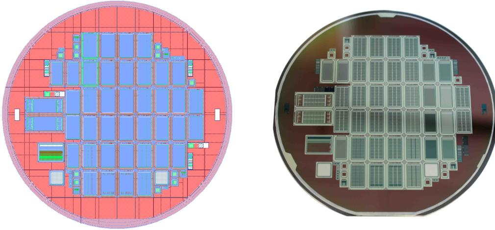
**Figure 5.7.:** The PS-p light prototype wafer. On the left: output of the design file that is used to save the structures during the design phase. On the right: final wafer produced at CiS.
