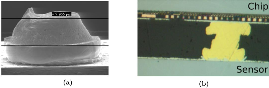
**Figure 5.16.:** Scanning electron microscope image of a gold-stud (a). The plateau at the bottom of the stud indicates the edge of the capillary. The small remnant at the top left of the stud is created when the capillary shears of the wire from the stud [Jun14]. Cross section of a bump-bonded assembly (b). The gold-studs are well aligned to each other and form a strong interconnection.
