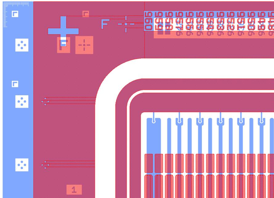
**Figure 8.2.:** Edge aluminum layers of a PS-p (blue) and PS-s (red) on top of each other. The bias and guard ring lie perfectly on top of each other, leading to the exact same active area of both sensors. The PS-p is  $600\ \mu\text{m}$  longer on its long side than the PS-s, exposing both edges and their alignment marks simultaneously.
