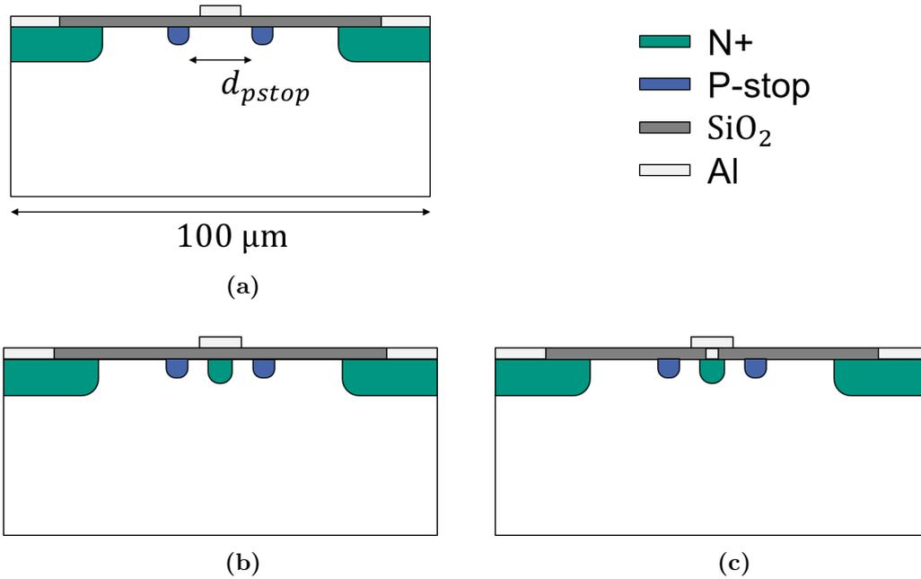
**Figure 7.3.:** Cross-sections of three bias rail geometries used during the simulation. Three different approaches are investigated: the reference design, which only includes a grounded aluminum rail on top of the silicon dioxide (7.3a), one design with a floating  $n$ -doped implant below the aluminum rail (7.3b) and a sensor with a connected implant which is set to ground potential by the aluminum rail (7.3c).
