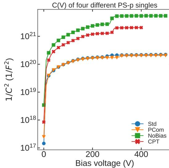
**Figure 9.11.:**  $C(V)$  measurements of the PS-p single sensors. The full-depletion voltage is hardly visible and can only be guessed between 150 V to 200 V bias voltage. The second step towards lower capacitances is independent of the sensor design and appears in all measurements. The total capacitance of the individual sensors is dominated by the number of PTS that are connected to the bias grid.
