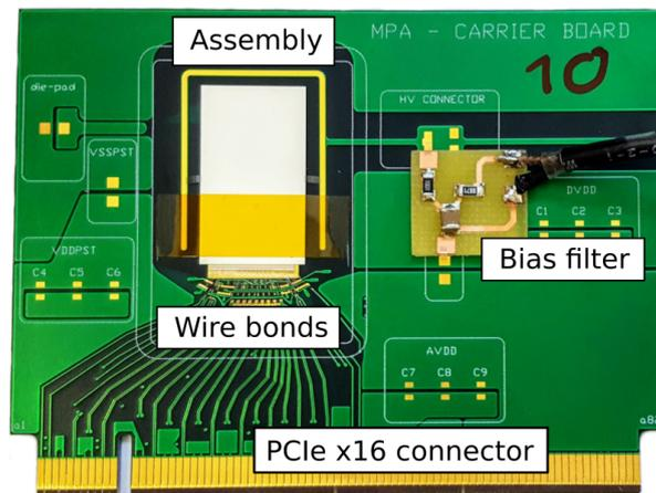
**Figure 10.5.:** Picture of the Single MaPSA on a carrier PCB. The assembly is placed with the sensor backside facing upwards on a gold-plated ground pad and fixed with a polyimide tape. Each I/O pad of the MPA is wirebonded to its dedicated traces on the PCB, which is routed to the PCI-e connector. The sensor backside is wirebonded to a U-shaped bias contact that is connected to the external power supply through a low-pass filter for noise reduction.
