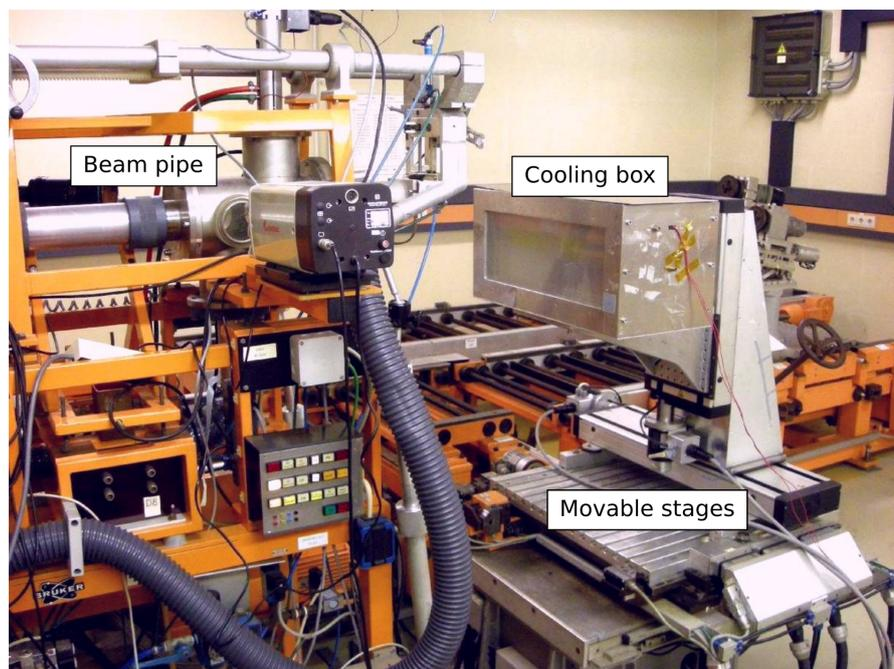
**Figure 10.25.:** The irradiation facility at the Zyklotron AG (ZAG) in Eggenstein-Leopoldshafen. The protons that come from the Kompaktzyklotron (KAZ) exit the beam pipe from the left. The samples are mounted on a frame that is placed inside the cooling box, which is flushed with dry air. The box is mounted on multiple stages to move the box inside the beam for a homogeneous irradiation of one or multiple samples [Ins19].
