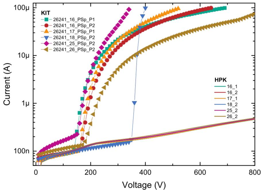
**Figure 9.1.:**  $I(V)$  measurements of several full-size PS-p sensors. Almost all measurements performed at KIT after dicing show an early breakdown below 200 V bias voltage. Only the sensor 18\_2 can be operated at 300 V, but does not reach by far the breakdown strength measured by Hamamatsu before the wafer was cut into single dice.
