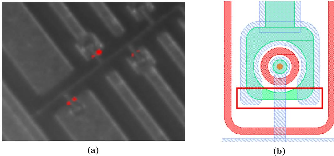
**Figure 9.14.:** Close-up view of a PTS during the infrared image analysis. Each PTS shows two spots of a high current density (a). These local breakdowns appear close to the bias rail extension of the PTS and the crossing points of the aluminum layer (b, blue) and the pixel implants (b, green), which is marked with a red box.
