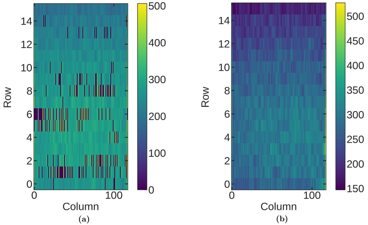
**Figure 10.9.:**  $\text{Sr}^{90}$  hitmap of two Single MaPSAs. The first few assemblies (a) show a significant number of dead pixels that are most likely related to uneven gold-stud bumps on the chip or/and the sensor. However, the majority of assemblies show no or only few missing bump bond connections (b).
