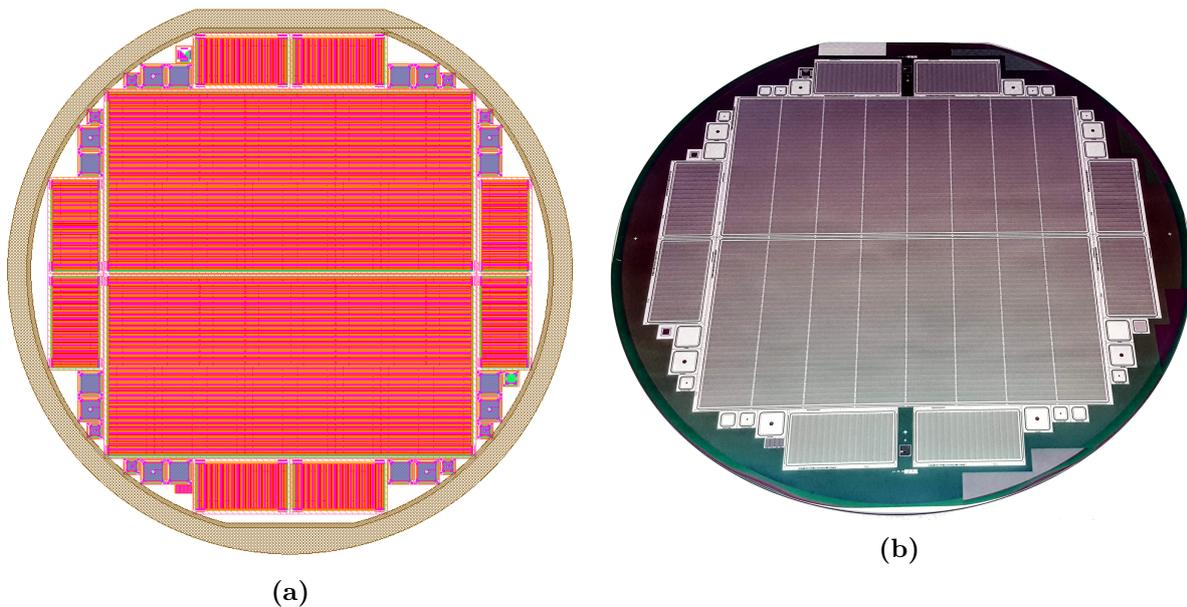
**Figure 8.1.:** The final GDS output file (a) and the processed PS-p wafer (b). Hamamatsu made some final changes to the proposed wafer layout, which are reflected in the additional space between some single sensors as well as some additional test structures.
