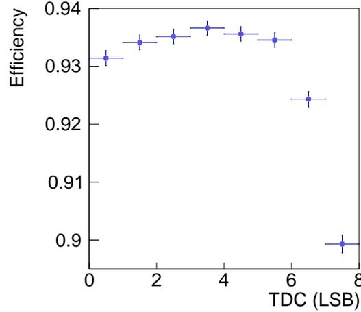
**Figure 10.26.:** Efficiency of an irradiated assembly at different TDC values in level sensitive mode. The efficiency varies strongly within a clock cycle due to the reduced signal height in irradiated sensors and the resulting shorter time period in which the signal stays above the threshold.
