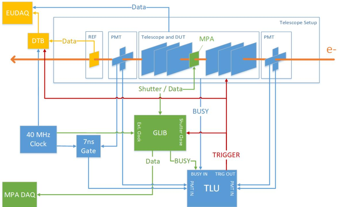
**Figure 6.8.:** The MaPSA light test beam readout and trigger schematics. One of the PMTs of the telescope is set in coincidence with a 7 ns gate to maximize the efficiency of the CMS Pixel timing reference (REF). The MaPSA light (green) stores its data locally and is not connected to EUDAQ which collects the data of the telescope (blue) and the reference plane (yellow).
