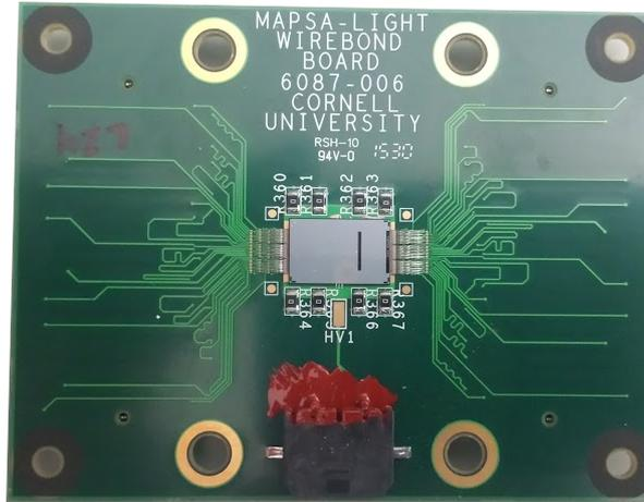
**Figure 5.18.:** Fully equipped MaPSA light wire bonded to its carrier board. The two high pin count connectors on the backside are only indicated by two guiding holes on the left and on the right end of the PCB. Three MPA-Lights are routed to one of these two connectors. The black terminal at the bottom serves as high voltage connection for the sensor, whose upward facing backside is wire bonded to the connected high voltage pad (HV 1) next to the assembly.
