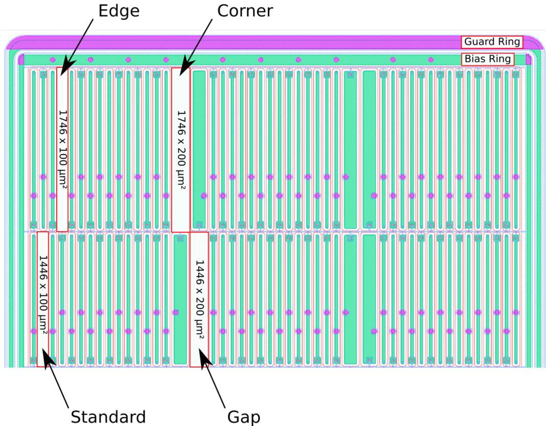
**Figure 5.8.:** Two rows of the PS-p light standard layout. Pixels in the first and last row are 300 μm longer than all the other pixels on the sensor. Four columns of gap pixels are widened to cover the space between two adjoining readout chips. The whole pixel matrix is surrounded by a bias and guard ring and enclosed by the sensor edge (not shown).
