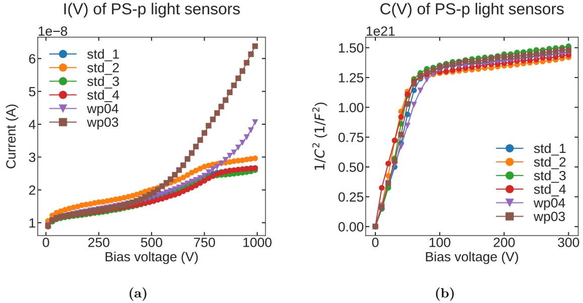
**Figure 5.11.:** I(V) (a) and C(V) (b) characteristics of six PS-p light sensors. All four PS-p sensors with the standard layout show no evidence of any failure up to a bias voltage of 1000 V. The two sensors with an increased width to pitch ratio of 0.3 and 0.4 on the other hand indicate a soft breakdown which is still within the exclusion limit set by the Outer Tracker community. All six sensors, regardless of their design are fully depleted at a bias voltage of about 80 V.
