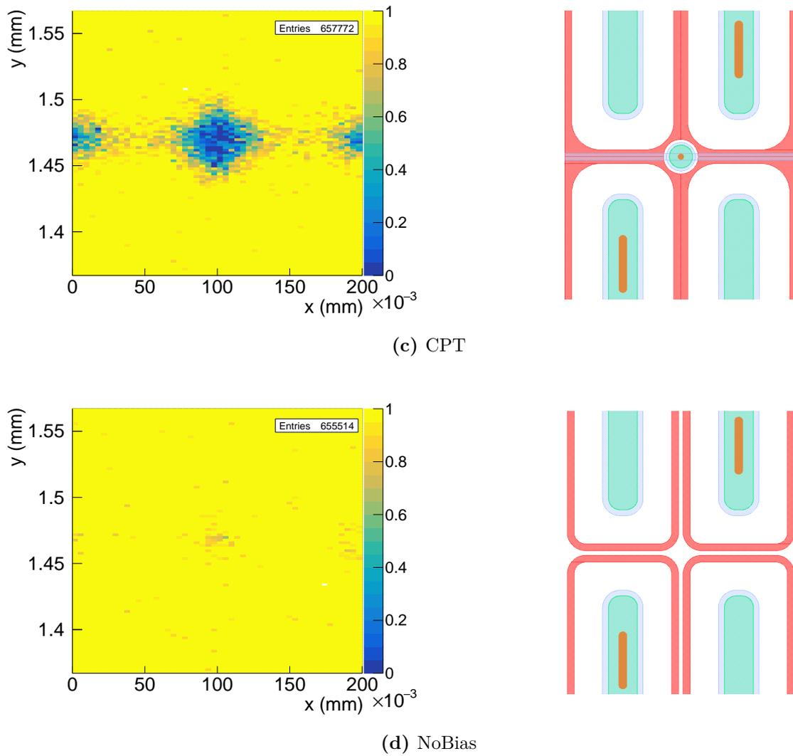
**Figure 10.18.:** Zoomed modulo efficiency maps of two Single MaPSAs equipped with a NoBias or CPT single PS-p sensor at a bias voltage of 200 V and a threshold of 110 LSB. Substituting four PTS with one CPT or omitting the bias grid completely (NoBias) increases the efficiency of the sensor significantly compared to the Standard layout.
