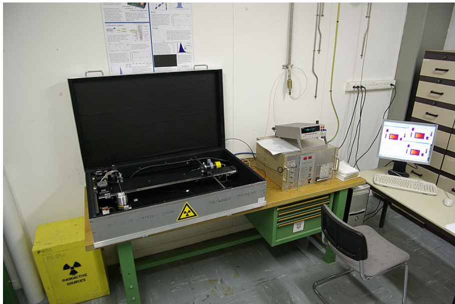
Figure 4.1: The Sr90 laboratory consists of the light-tight scanbox, control crate, multimeter and data acquisition PC [42].
