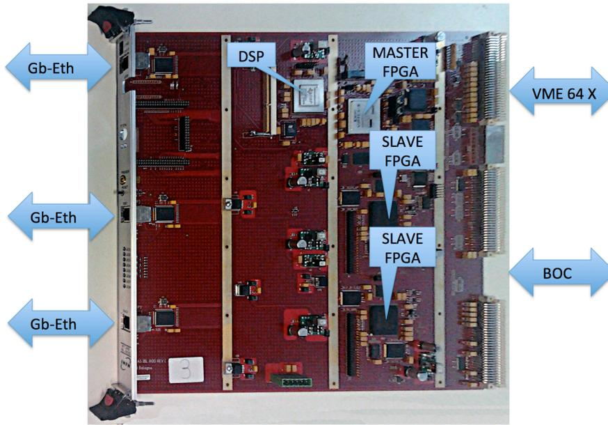
Figure 2. A picture of the revision D ROD-card.
