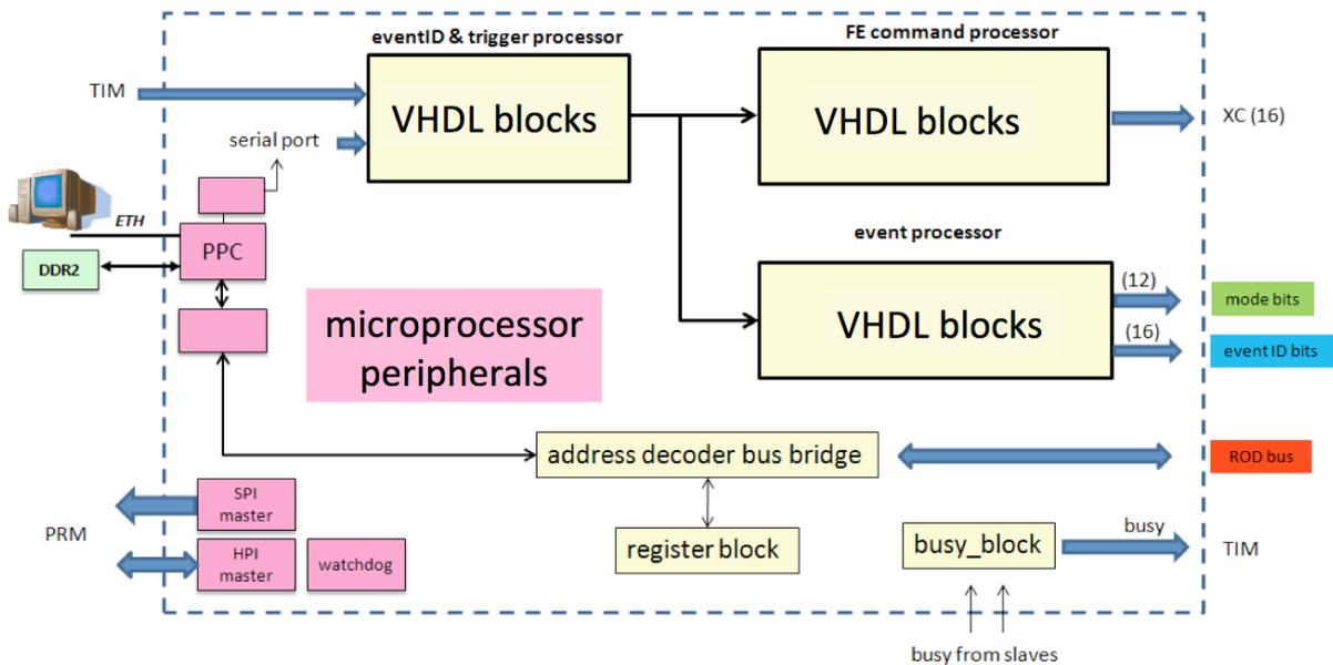
Figure 3. The BOC-ROD master firmware logic view.
