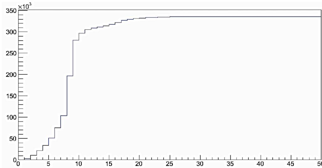
Figure 6. Threshold scan run from the Console: s-curve from all pixels in the chip in one plot.
