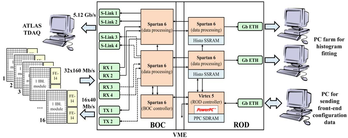
Figure 1. The IBL readout electronics layout.
