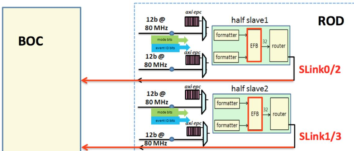
Figure 4. Data taking with 32 FeI4 emulators per BOC-ROD.
