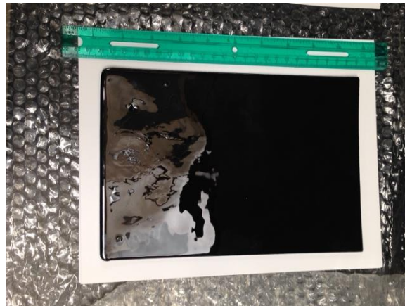
Figure 5. Photograph of a semi-conductive glass plate as produced by COE College (Iowa). The bulk resistivity was measured to be approximately 10^{10} \Omega\text{cm} .
