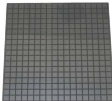
Figure 27: Photograph of the Silicon wafers produced by Hamamatsu. This wafer contains 324 pixels.
