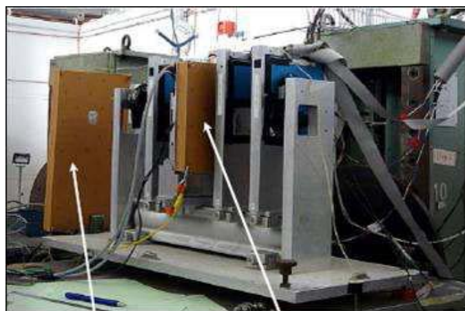
Figure 37: The setup used for the beam-test. The three planes of silicon strip detectors are inside the aluminum frames. The sensor plane under test is mounted inside the copper-colored PCB box between the second and third aluminum frame.
