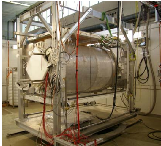
Figure 15: Movable stage around the magnet PCMAG in DESY's test beam area T24/1.
