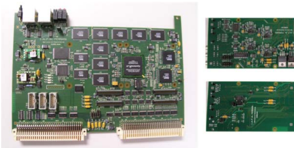
Figure 7: The EUDRB (left), and the analogue (upper right) and digital (lower right) daughter cards
