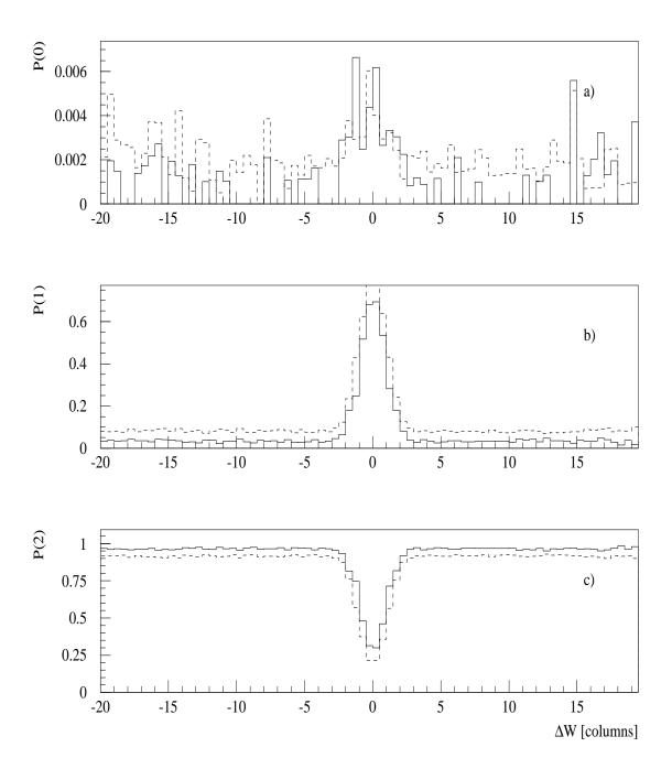
Figure 4: Probability to find 0 (a), 1 (b) or 2 (c) hits in the region where two tracks point out for W-plane of fiber detector. Probabilities are shown as function of estimated coordinate difference of pair at the W-plane by solid line for experimental data and dashed line for simulation.
