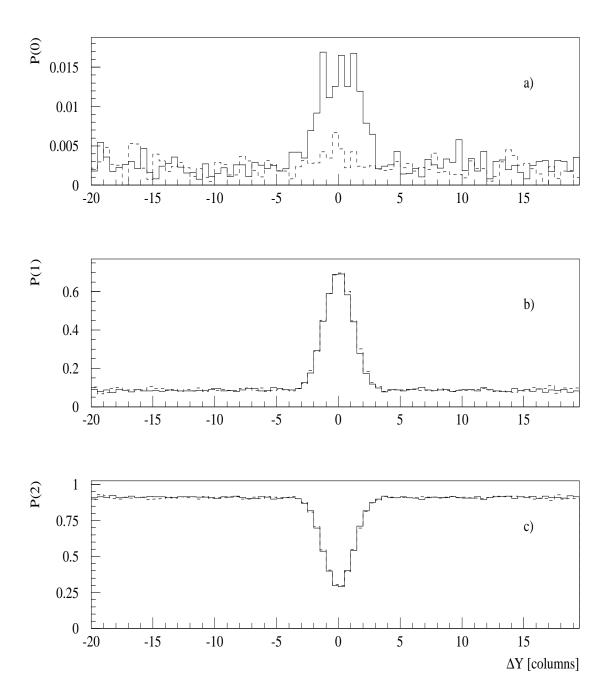
Figure 3: Probability to find 0 (a), 1 (b) or 2 (c) hits in the region where two tracks point out for Y-plane of fiber detector. Probabilities are shown as function of estimated coordinate difference of pair at the Y-plane by solid line for experimental data and dashed line for simulation.
