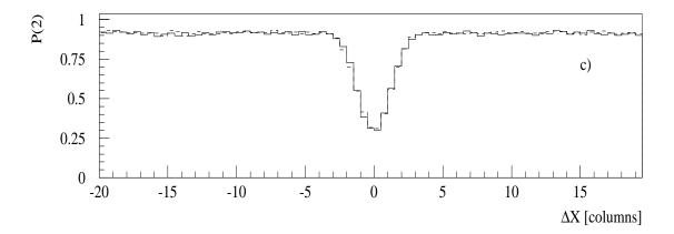
Figure 2: Probability to find 0 (a), 1 (b) or 2 (c) hits in the region where two tracks point out to the X-plane of fiber detector. Probabilities are shown as function of estimated coordinate difference of pair at the X-plane by solid line for experimental data and dashed line for simulation.
