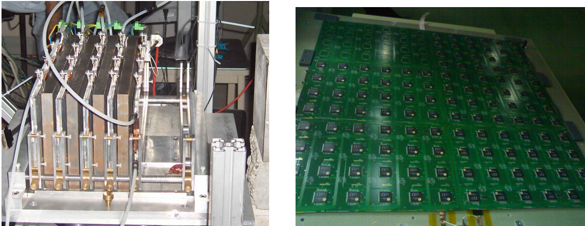
FIGURE 4.4-22. Mini-DHCAL prototype (left); Prototype of a large instrumented GRPC (right).
