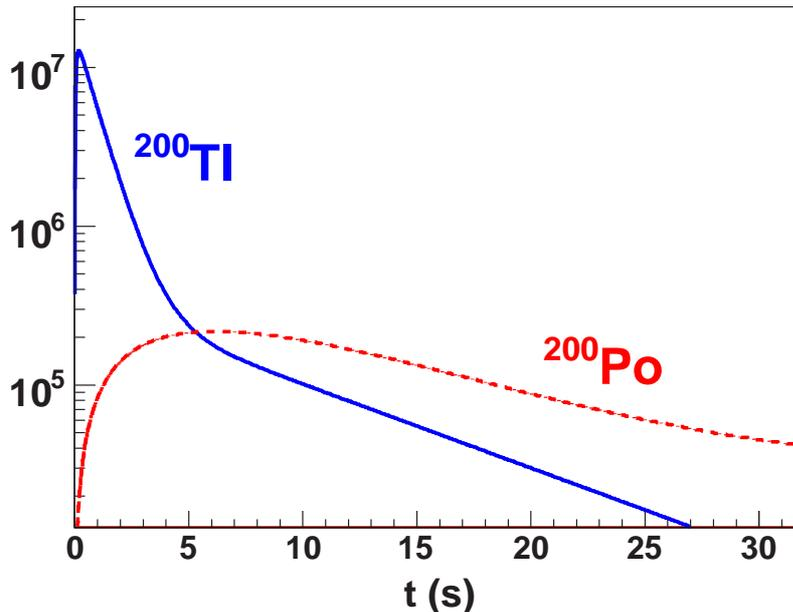
FIG. 2 –  $^{200}\text{Po}$  and  $^{200}\text{Tl}$  release curves from [30], considering one proton pulse of  $N_p=2\times 10^{13}$  only; where  $t$  corresponds to the time since proton impact.
