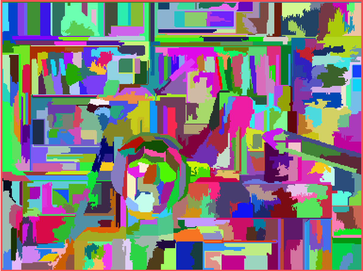
Figure 4.4: Segmentation of the left image in the Tsukuba data (Nakamura et al., 1996) using mean-shift algorithm.
