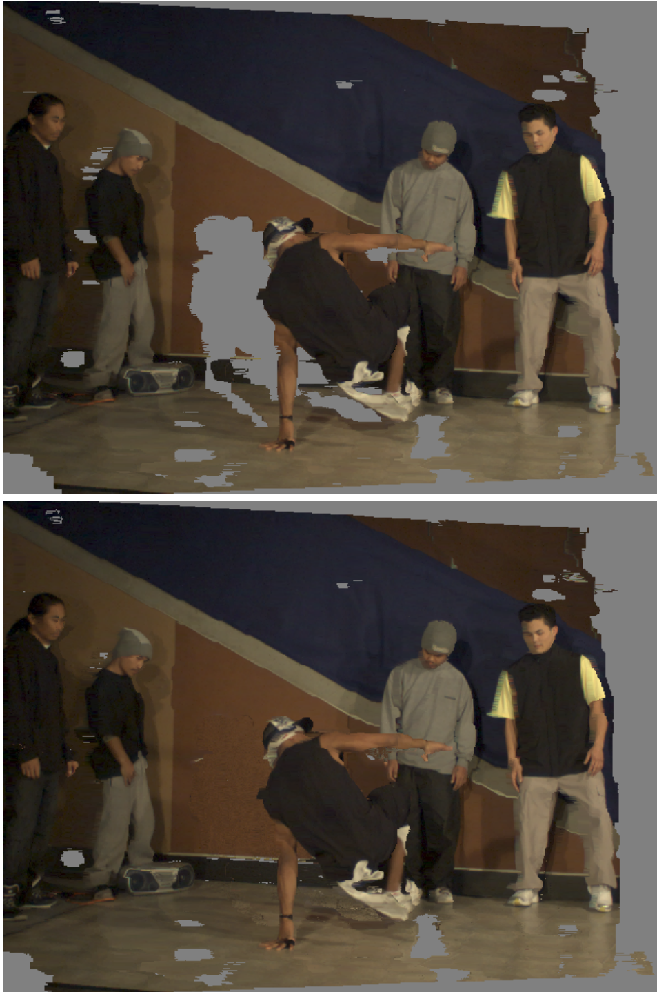
Figure 7.9: The first image is a pure reprojection, leaving holes due to the depth map being 2D for a camera at a different location. The second image is the same reprojection, but the holes are filled by the background model which is information available from the BiasedBP algorithm.
