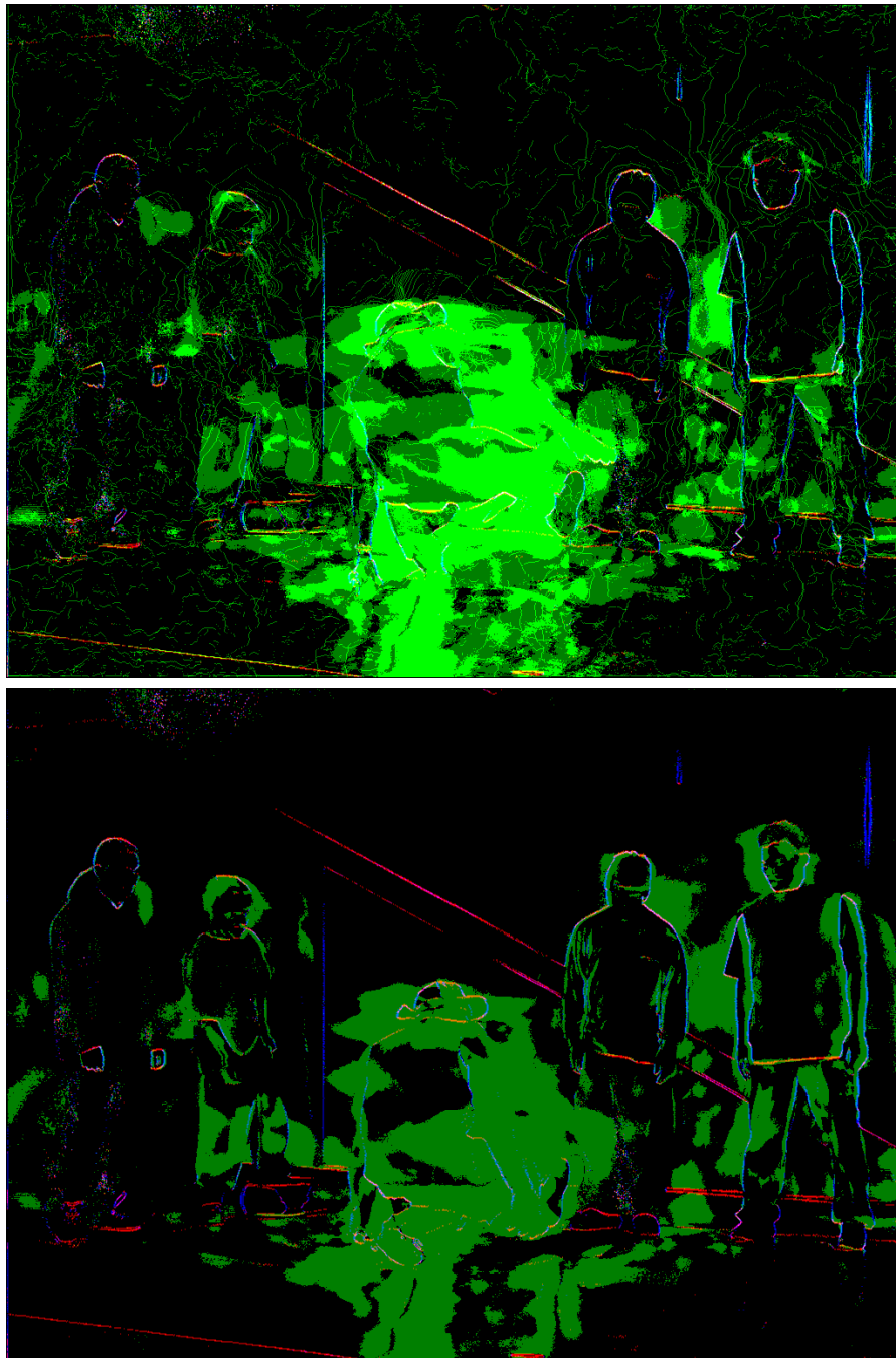
Figure 5.3: Visualizations of Robust Temporal Belief Propagation in detail, for the second frame of the breakdancer sequence. The top image uses no optical flow (e.g. straight through, assumes no motion), while the bottom uses the optical flow algorithm of (Proesmans et al., 1994). The non-black pixels indicate which neighbor nodes are disconnected by my robustness algorithm. Observe that less temporal neighbors are disconnected with a better optical flow estimate.
