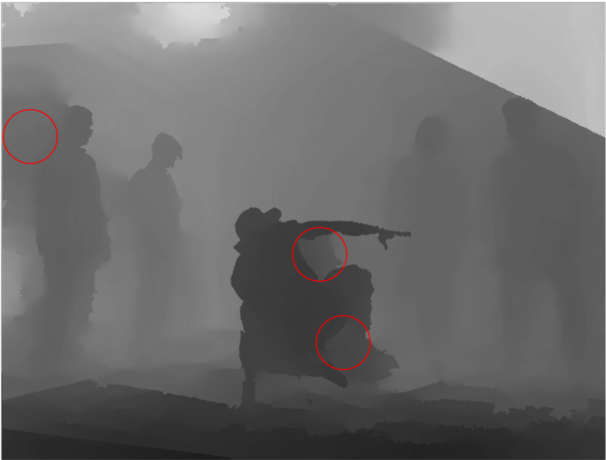
Figure 4.1: State of the art depth map for breakdancers (Zitnick et al., 2004) showing regional artifacts caused by occlusions. Some specific ones are highlighted with red circles. Note that (Zitnick et al., 2004) focused on video quality and not correct depth values.
