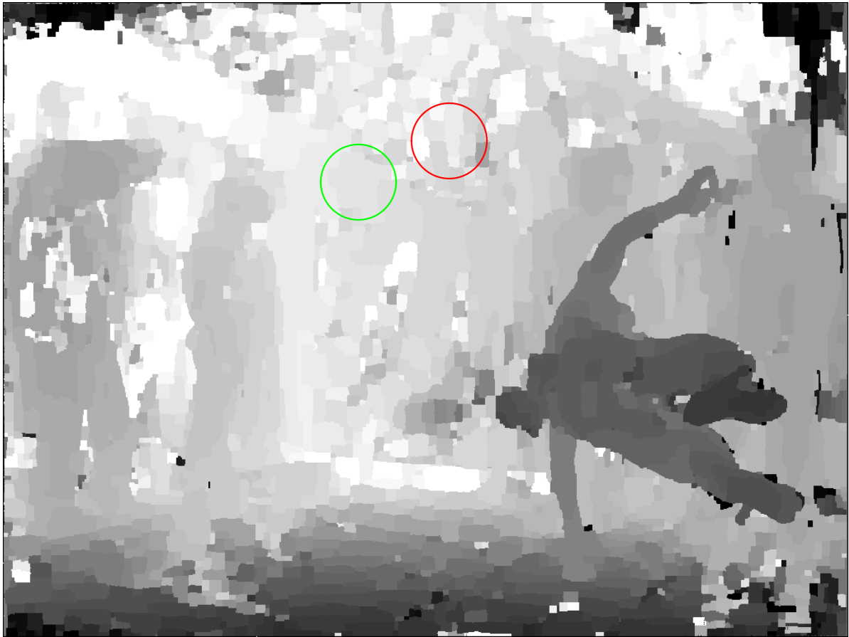
Figure 6.7: Depth map using regular BP. Notice the limited spatial influence of the features along the diagonals on the back wall (the green circle highlights one example). Compare this to the mottled effect seen in the near-uniform regions, as in the red circle.
