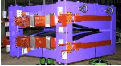
Figure 5: "Return-Yoke Free" Magnet for 150MeV FFAG accelerator.
