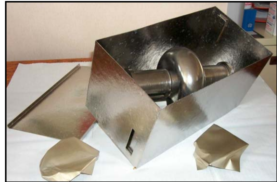
Figure 6 : The Titanium box shields the cavity from the furnace atmosphere during the heat treatment.
