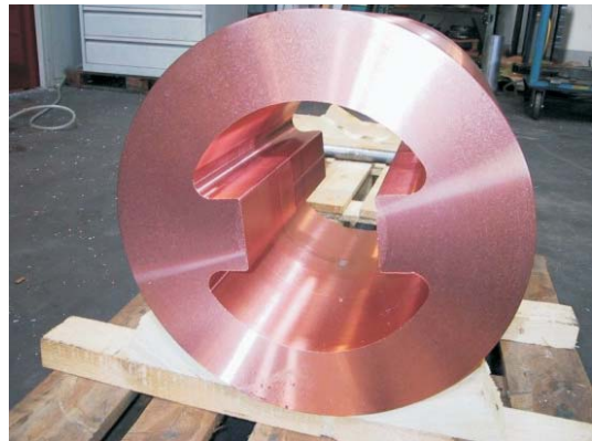
Figure 7: The picture shows the one of the central module after the first machining procedure.
