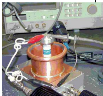
Figures 10, 11, 12: Circuit diagram, Frequency response of the divider, and photo under measurement, where 5pF/18kV capacitor is installed at the center of the guard ring
