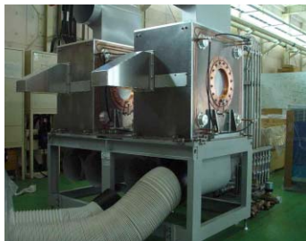
Figure 4 Accelerating system under construction.
