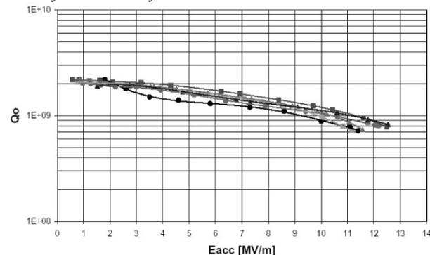
Figure 5: Summary of test results on 500 MHz single cell cavities of the Cornell design. All cavities show similar behaviour during RF test showing the reliable preparation procedure.
