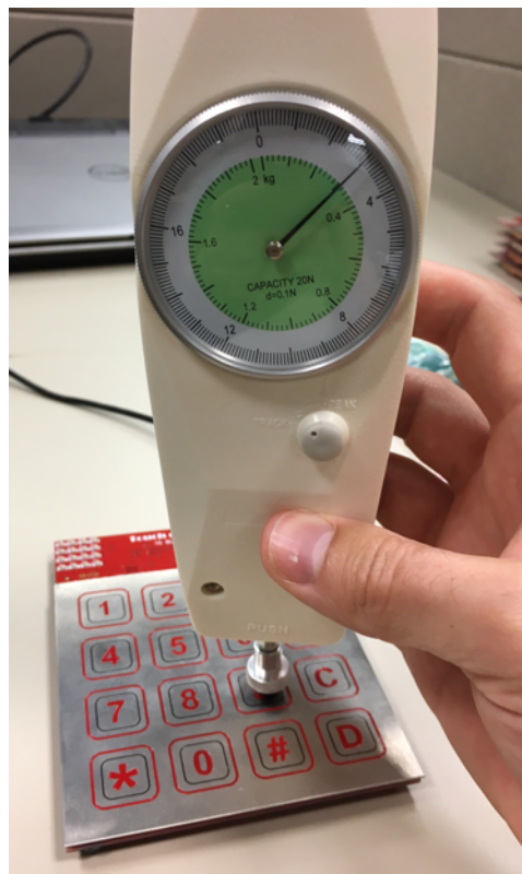
图 32. Test Setup With Newton Meter to Check TIDA-01102 Response to Known Forces
