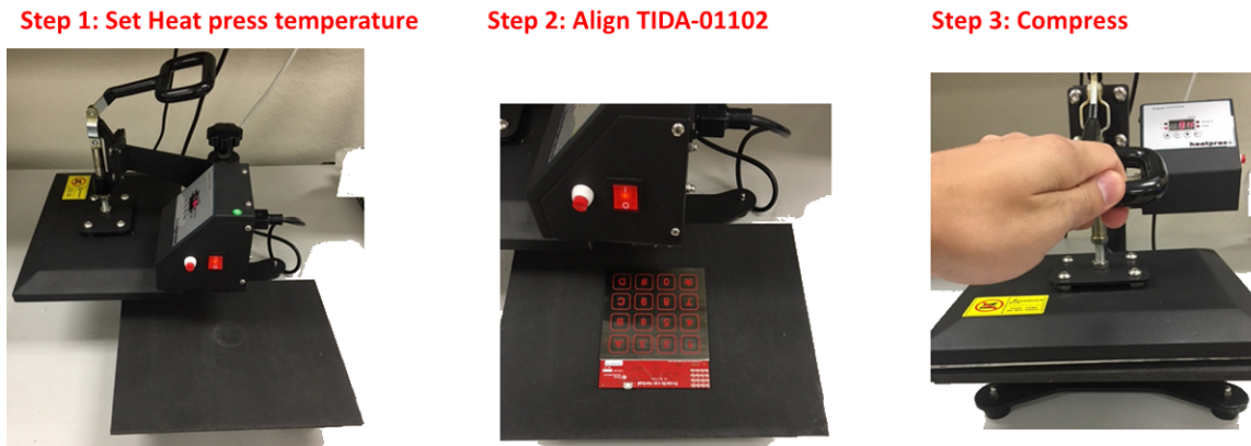
图 31. Example Compression Technique Using Heat Press
