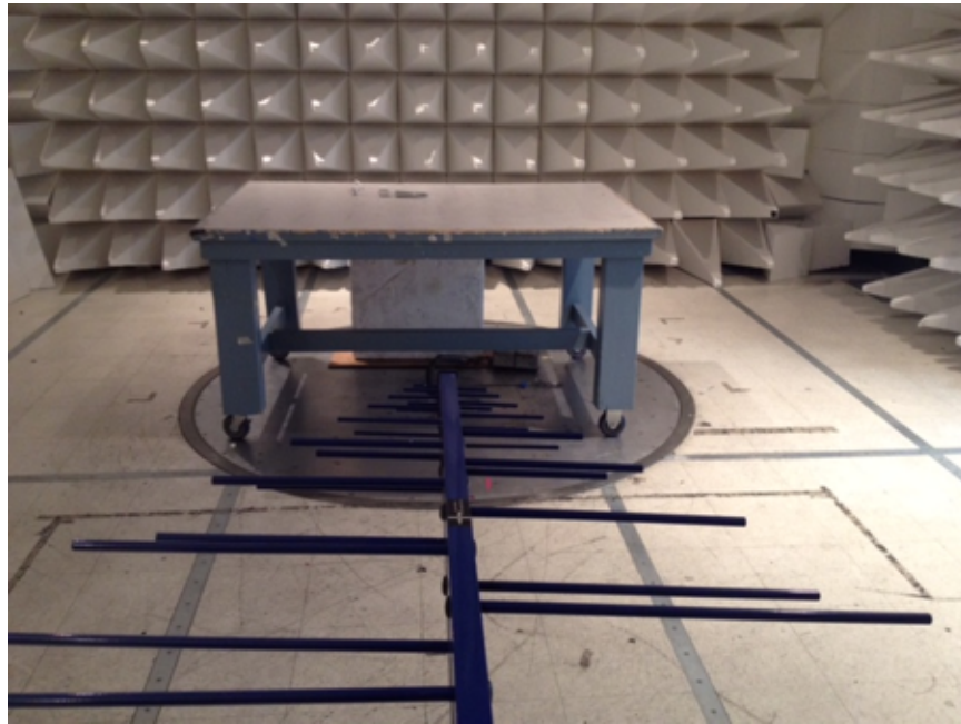
图 43. EMI Setup for CISPR22 Emissions Testing
