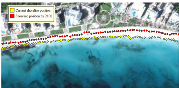
Figure 17. Present-day shoreline position (in black) and landward migration (in red) in the worst case scenario (mean sea level rise under RCP85 and extreme wave conditions) by the end of the 21st century in the Cala Millor beach.
