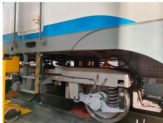
Figure 5. Instrumented wheelset detection system.
