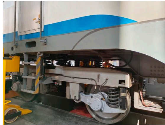
Figure 5. Instrumented wheelset detection system.
