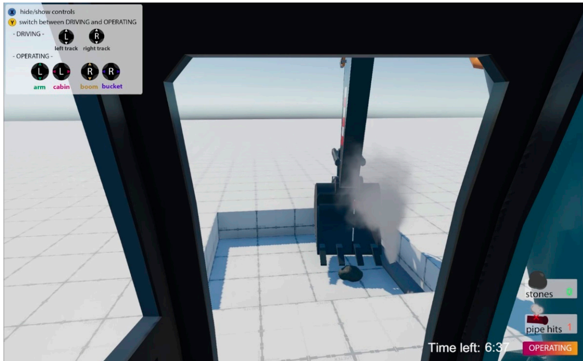
Figure 3. A scene from the training process: the user is trying to dig out the stone from the pit without cement liquid in it but has just hit the steam pipe.
