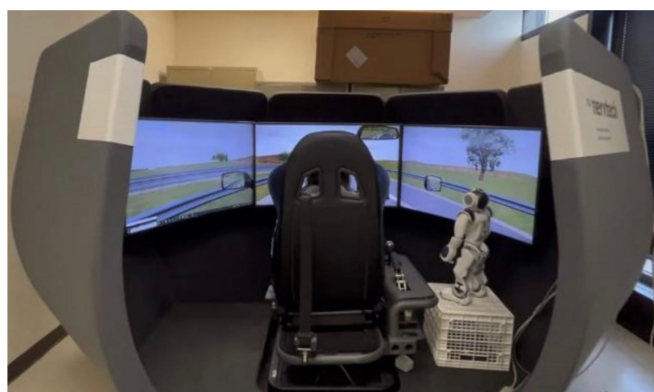
Figure 2. Experiment setup: Nervtech™ driving simulator with the IVIA.
