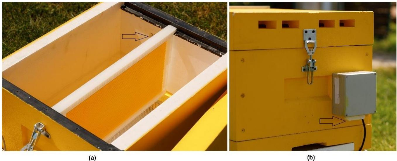
**Figure 4.** Smart hive sensors: (a) internal temperature and humidity sensor; (b) IoT block with external temperature and humidity sensor.
