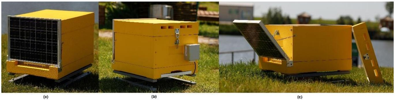
**Figure 2.** Smart hive: (a) front view, (b) back view, (c) exploded view.
