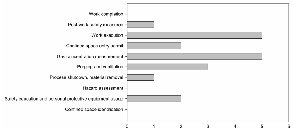
Figure 5. Pie chart showing the proportion of chemical accidents by confined-space work stage.
