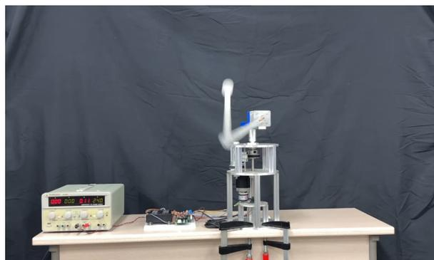
Figure 12. A YouTube video capture of the 12 transition controls of a rotary double inverted pendulum.
