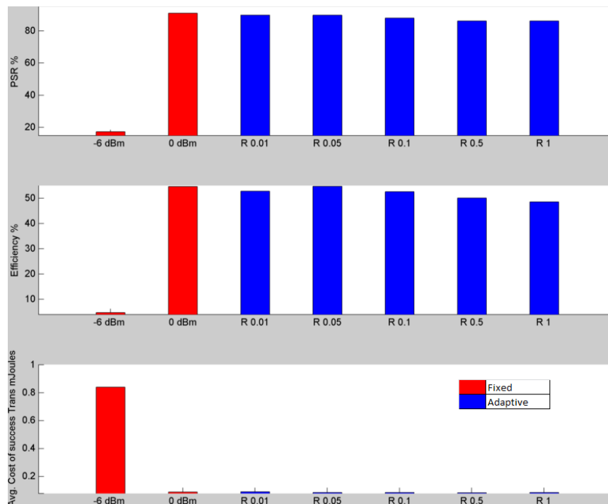
Figure 6. Comparison of the efficiency and average cost of successful transmission based on the PSR when the distance between the sensor and the hub is 24 m and collected during the busy hour. The minimum energy consumption of fixed power is achieved at 0 dBm, primarily because it has much higher PSR and efficiency than at -6 dBm. The adaptive protocol consumes 6% less energy than the fixed power transmission at 0 dBm when R = 0.5 . The efficiency of the fixed power transmission at 0 dBm is a touch higher than that of adaptive protocol at R = 0.5 .
