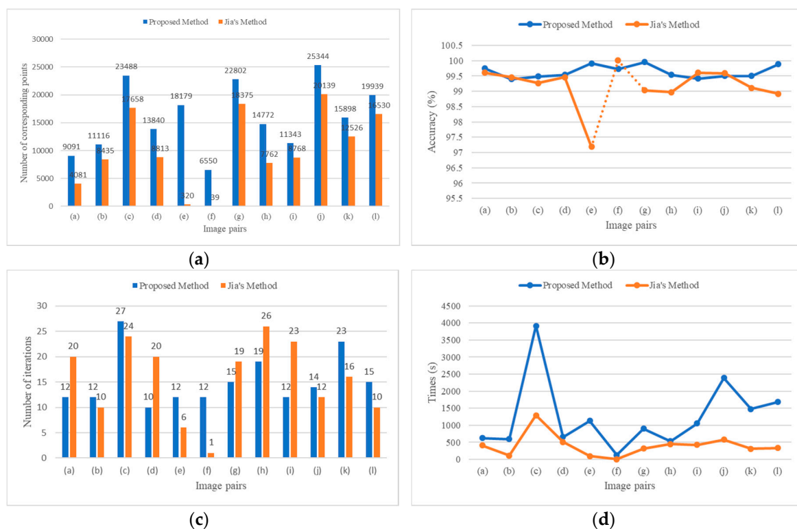
Figure 13. Comparison of the proposed method and Jia's method for 12 sets of image pairs: (a) number of matched points obtained by both methods; (b) accuracy of the two methods; (c) number of iterations of the two methods; (d) running times of the two methods.
