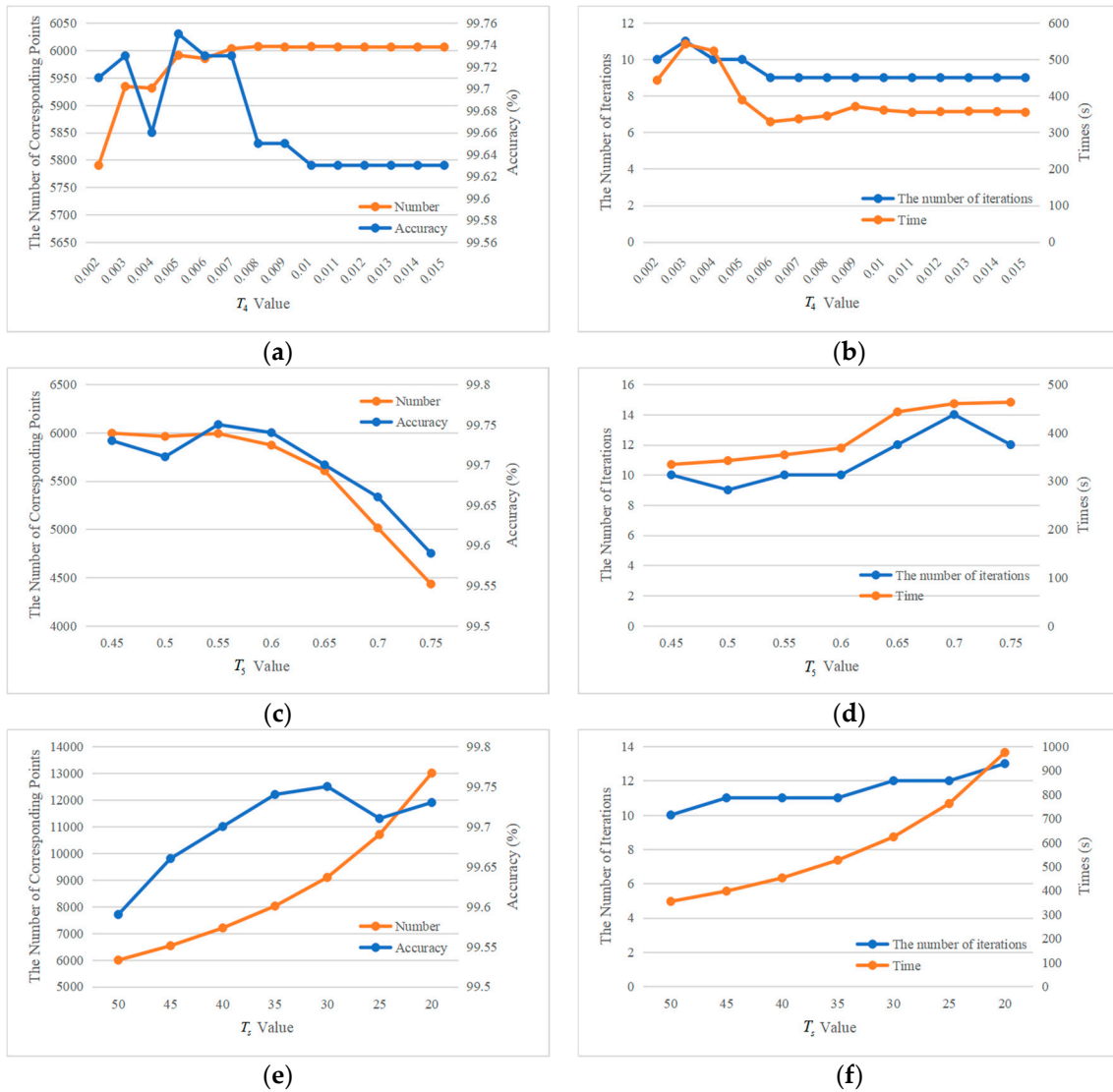
Figure 11. Matching results of different parameters: (a,c,e) represent the number of corresponding points and accuracy of matching; (b,d,f) represent the number of matching iterations and running time of the proposed method.
