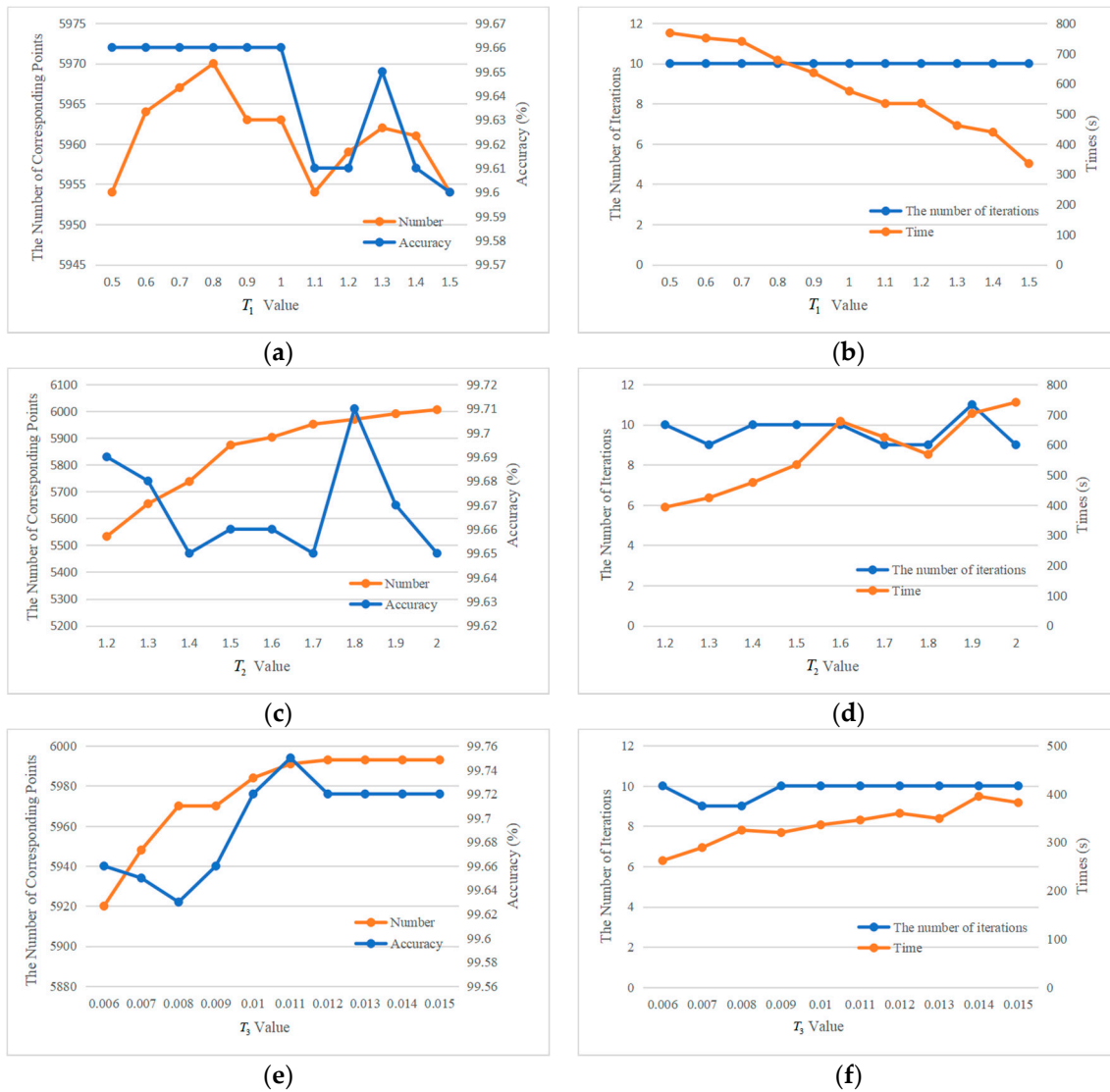
Figure 10. Matching results of different parameters: (a,c,e) represent the number of corresponding points and accuracy of matching; (b,d,f) represent the number of matching iterations and running time of the proposed method.
