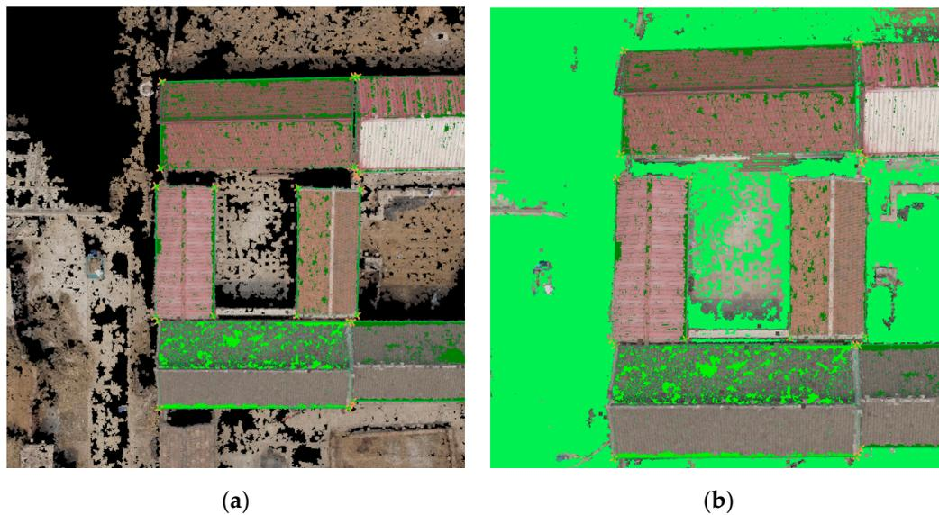
**Figure 4.** Images with manually drawn (a) upper building surfaces and (b) ground with a consistent level.
