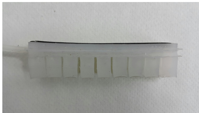
Figure 6. Completed soft pneumatic actuator with integrated MWCNT sensor.
