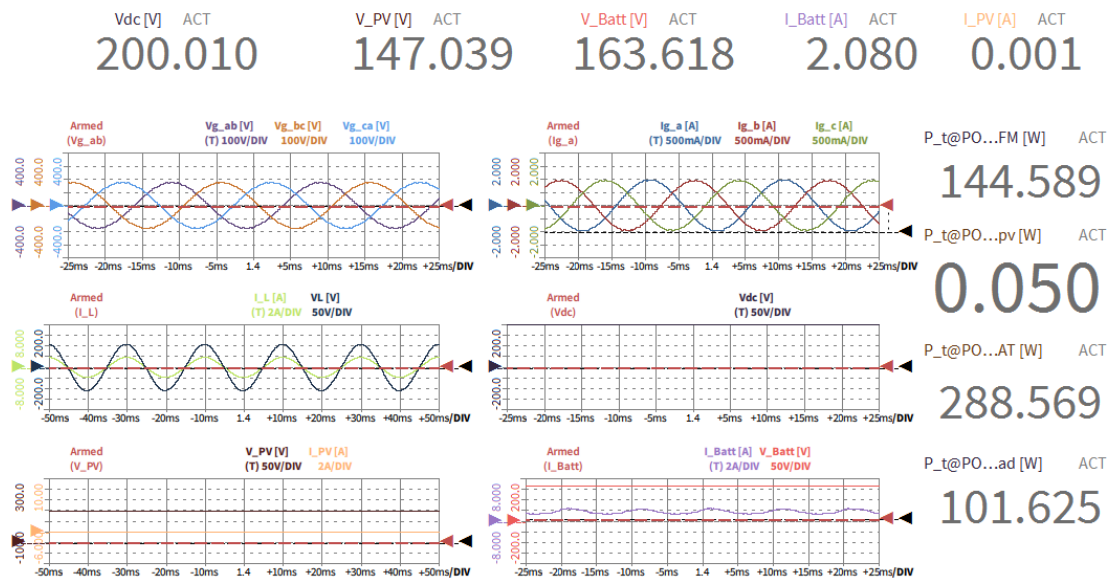
Figure 20. Only battery connected feeding to the dc-link.
