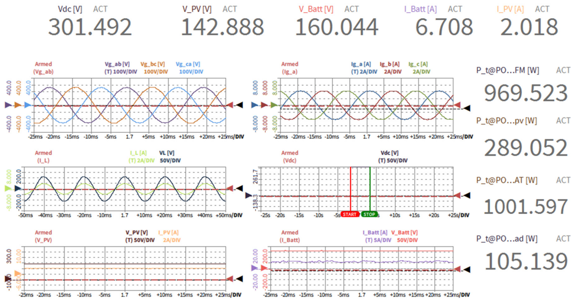
Figure 22. Battery and PV feeding into dc-link.
