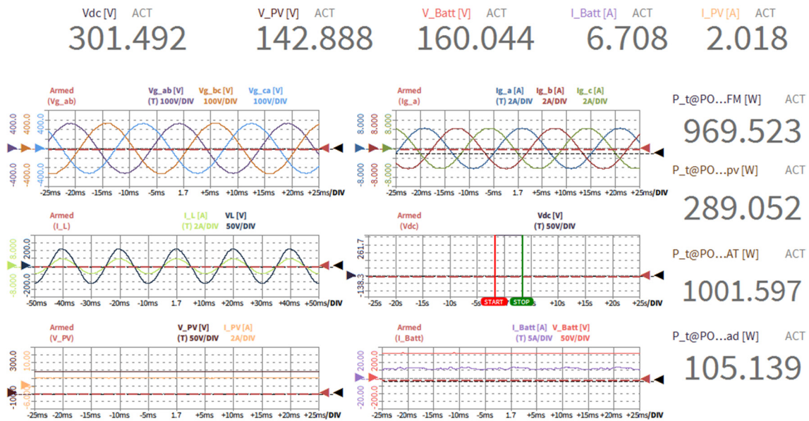
Figure 25. Increasing GFM voltage and DC-link voltage.
