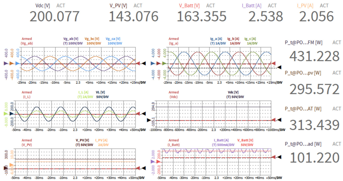
Figure 24. Balanced GFM with increased load.
