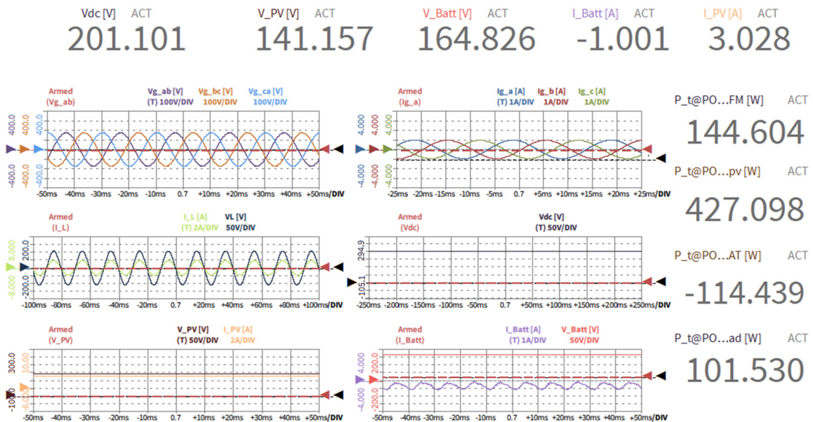
Figure 21. Excess energy is used to charge the battery.
