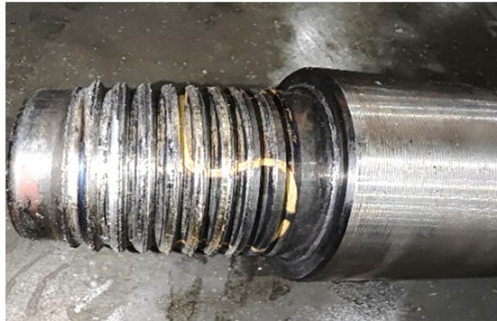
**Figure 1.** Bionic joint after wear.
