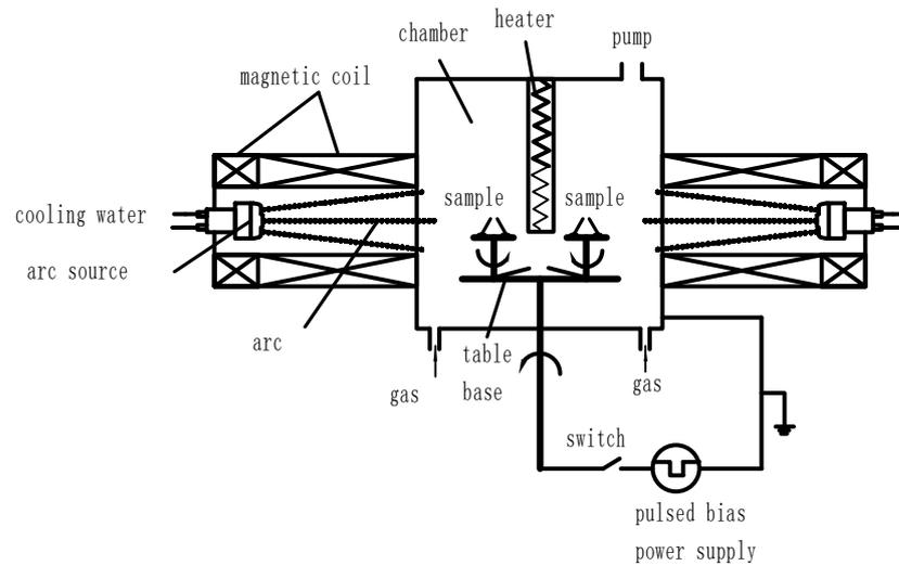
**Figure 3.** Principle of vacuum arc ion plating.
