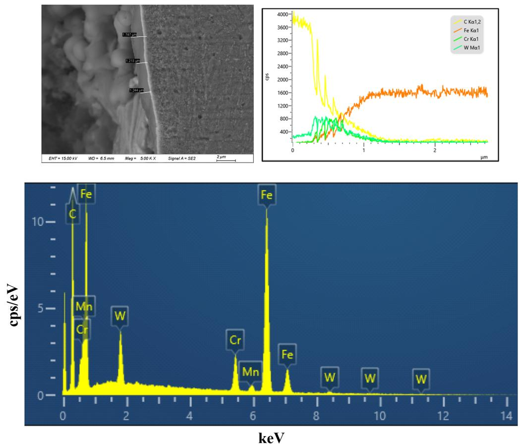
Figure 10. SEM and EDS analysis of diamond-like carbon films.
