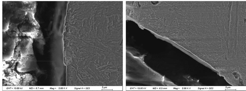
Figure 9. Surface of outer thread and inner thread after coating.
