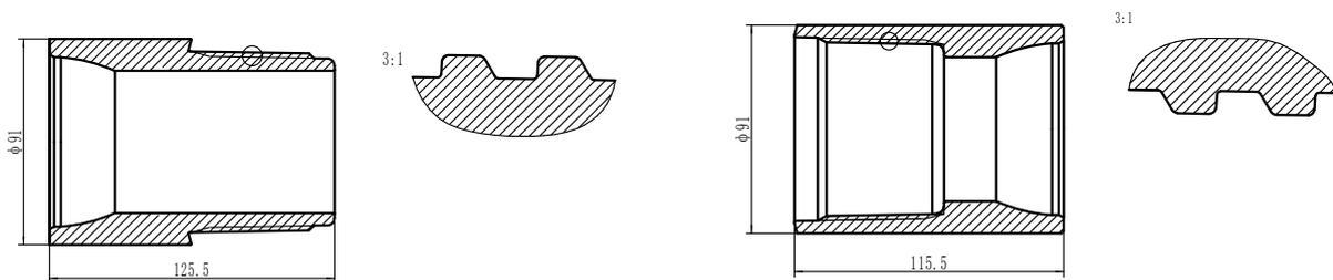
**Figure 4.** The  $\Phi 89$  mm joint structure.
