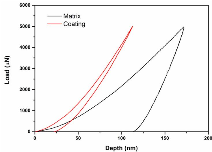
**Figure 6.** Nano-hardness test.
