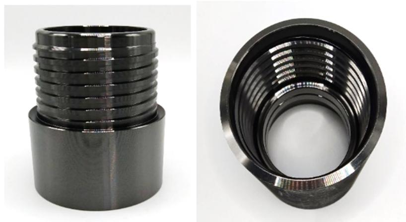
Figure 5. Joints after DLC coating.
