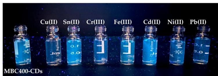
**Figure 6.** (a,b) is the selectivity test of the prepared MBC 400-CDs towards different metal ions, (c) a photo showing the MBC400-CDs sample before and after quenching using different heavy metal ions under irradiation using a longer wavelength UV lamp.
