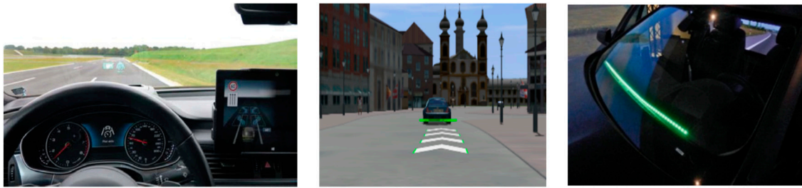
Figure 4. Most common visual HMI-elements used in aHMIs. (a) Instrument cluster, head-up display, and monitor in the center console used for presenting automation state and maneuvers [19]. (b) Augmented marking of a front vehicle and the control range in the head-up display [23]. (c) LED-strip in the windshield to visualize the automation mode using color-coding [21].
