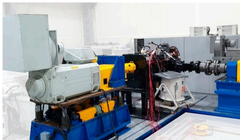
(b) photograph of the 3-axis dynamometer system
