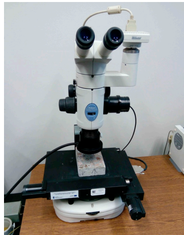
Figure 1. View of the microscope with the attachment mounted on the objective lens for additional illumination of concrete specimens.
