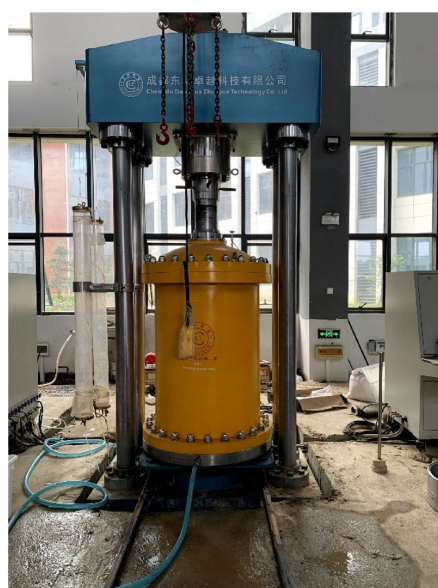
Figure 5. GSZ501 large triaxial compression tester for coarse-grained soil (size sample of \Phi 500 \times 1000 mm).
