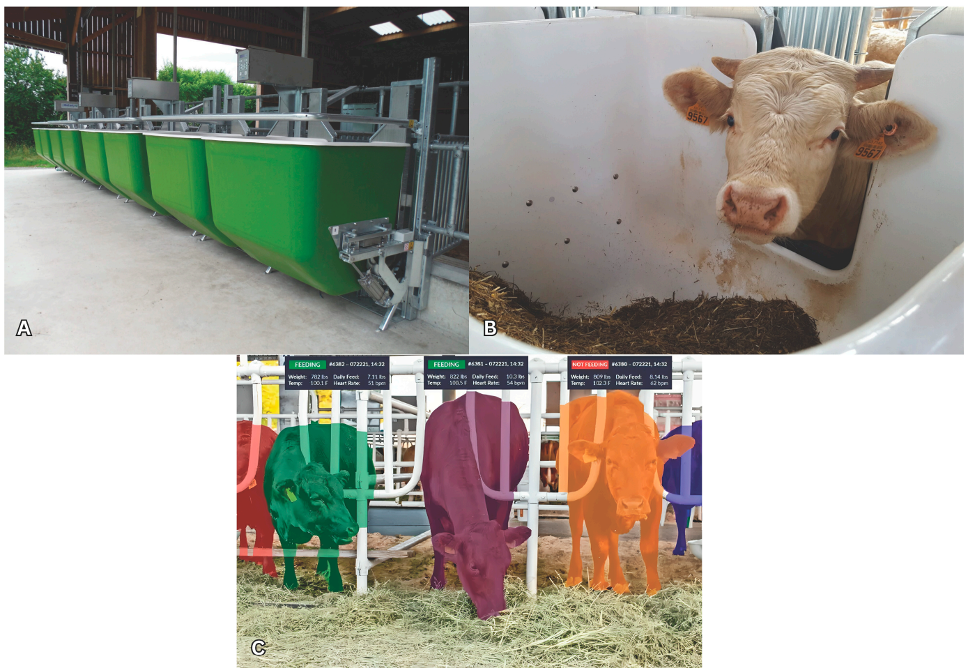
Figure 1. Example of equipment used to monitor and record feed intake in cattle. (A) The feeding lane is equipped with multiple electronic scales for individual feed intake monitoring—adapted from Biocontrol ( https://biocontrol.no/products-2/controlling-and-recording-feed-intake/ , accessed on 6 November 2024). (B) Close-up of a feed intake system with individual animal identification—copyrights sourced from Biocontrol ( https://biocontrol.no/products-2/controlling-and-recording-feed-intake/ , accessed on 6 November 2024). (C) Visual monitoring of feeding behavior using color-coded overlays on each animal to track feeding status and health parameters in real-time—copyrights sourced from Miguel Ángel Cabrera Miñagorri/Pipeless ( https://www.pipeless.ai/industries/cattle-raising , accessed on 6 November 2024).
