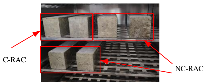
Figure 1. NC-RAC and C-RAC specimens.
