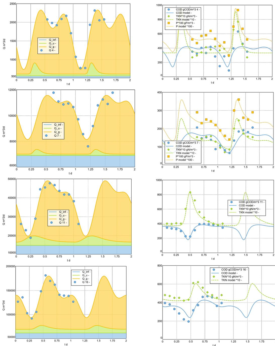
**Figure 11.** Reproduction of daily pattern, variant 2023 (selection). The legends for measured Q and measured COD include the id (1–21) of the analysed sample plant. See Appendix C for all analysed data sets.
