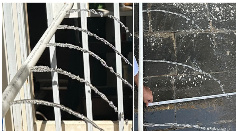
Figure 6. View of water jets issuing from the manifold and ports.
