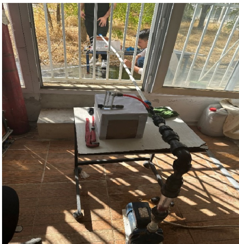
Figure 1. Test setup (pump, water flow meter, air-flow meter, Venturi device, and manifold).
